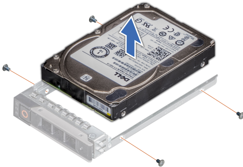
Figure 69. Removing the drive from the drive carrier
