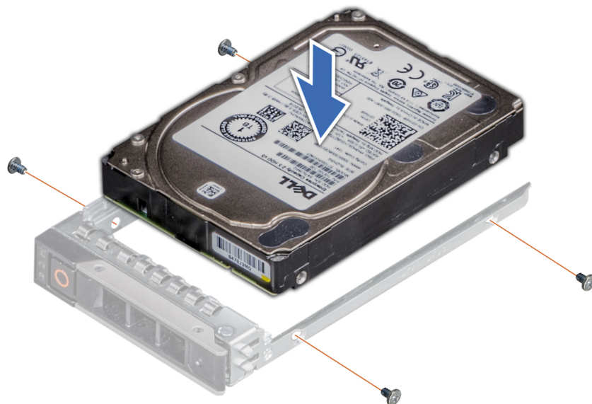
Figure 71. Installing a drive into the drive carrier
