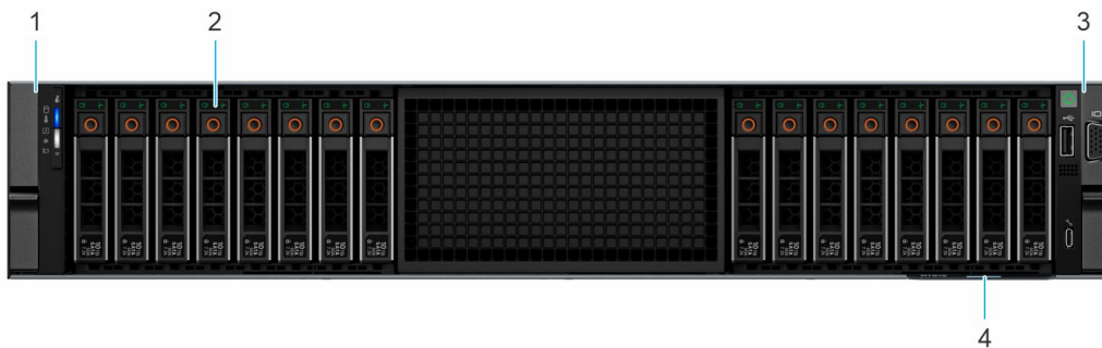
Figure 2. Front view of 16 x 2.5-inch drive system
