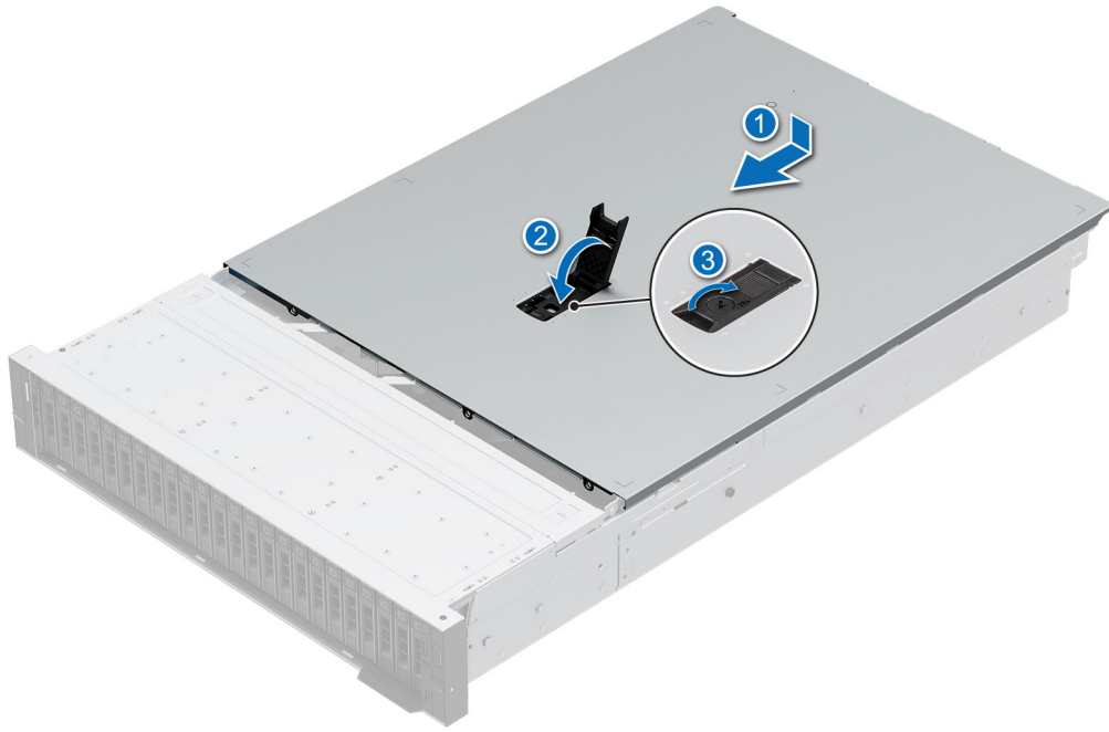
Figure 34. Installing the system cover
