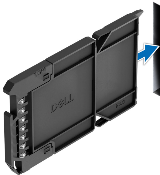
Figure 64. Installing an EDSFF E3.S drive blank
