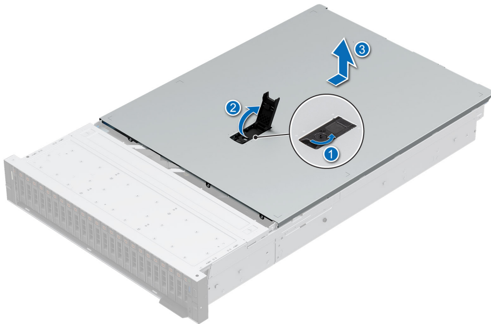
Figure 33. Removing the system cover
