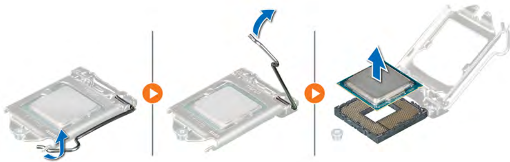
Figure 52. Removing the processor
