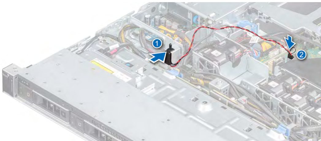
Figure 32. Installing the intrusion switch
