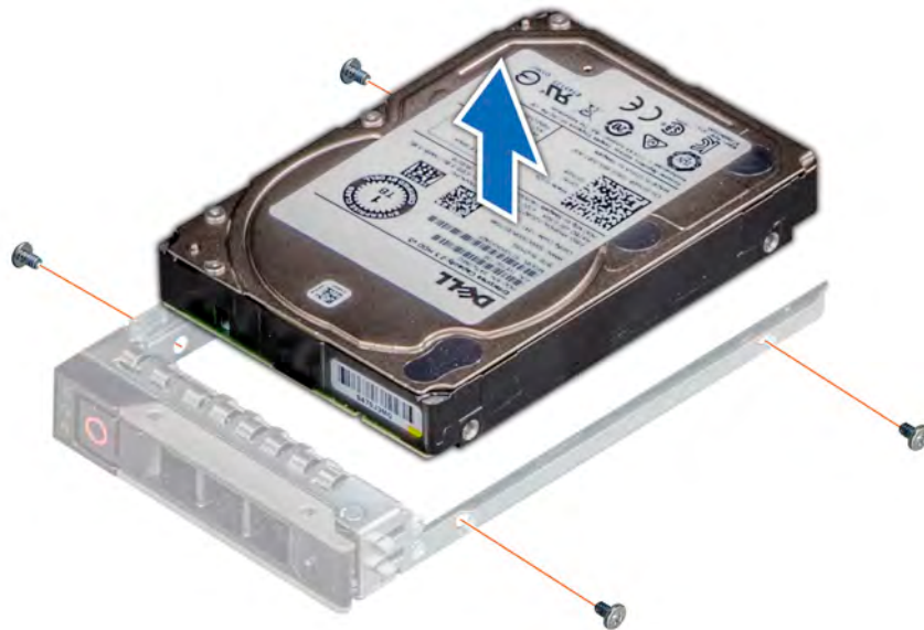
Figure 27. Removing the drive from the drive carrier
