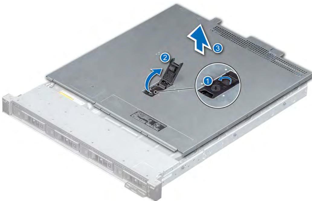
Figure 15. Removing the system cover
