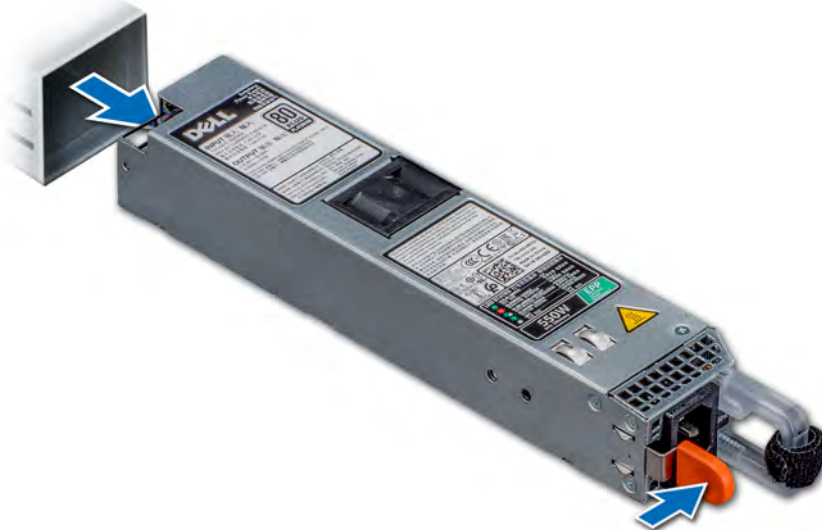
Figure 70. Removing a power supply unit
