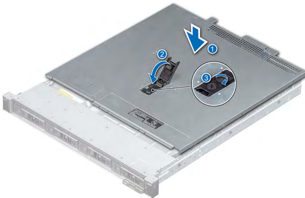
Figure 16. Installing the system cover
