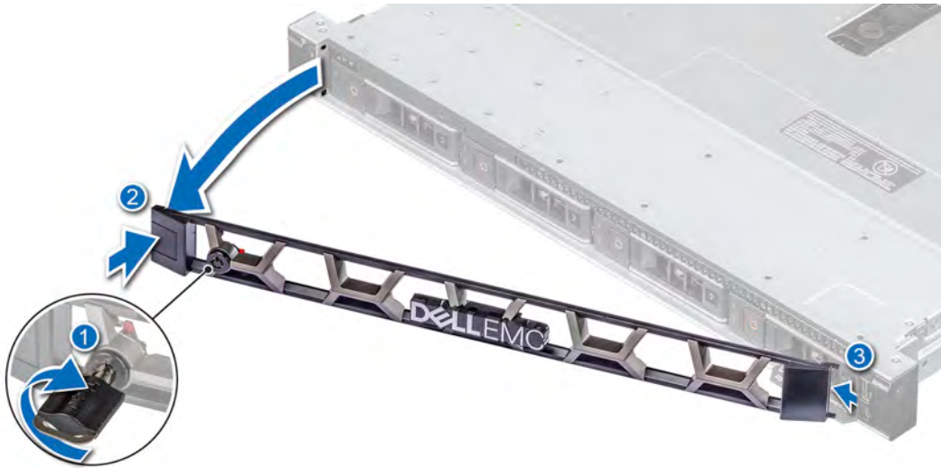
Figure 13. Removing the optional front bezel
