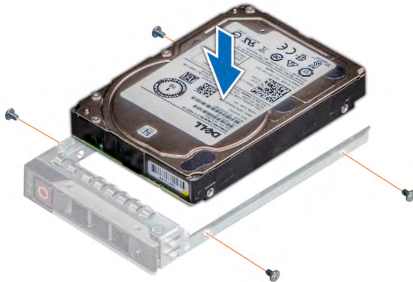
Figure 28. Installing a drive into the drive carrier
