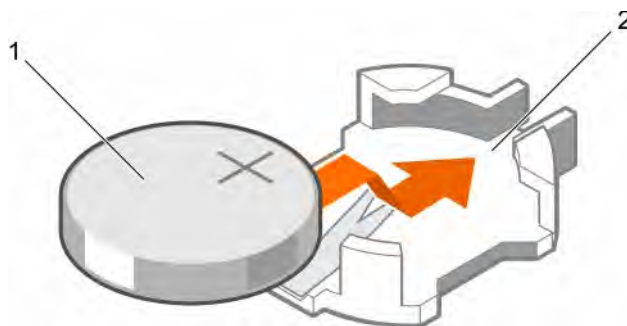
Figure 77. Installing the system battery
