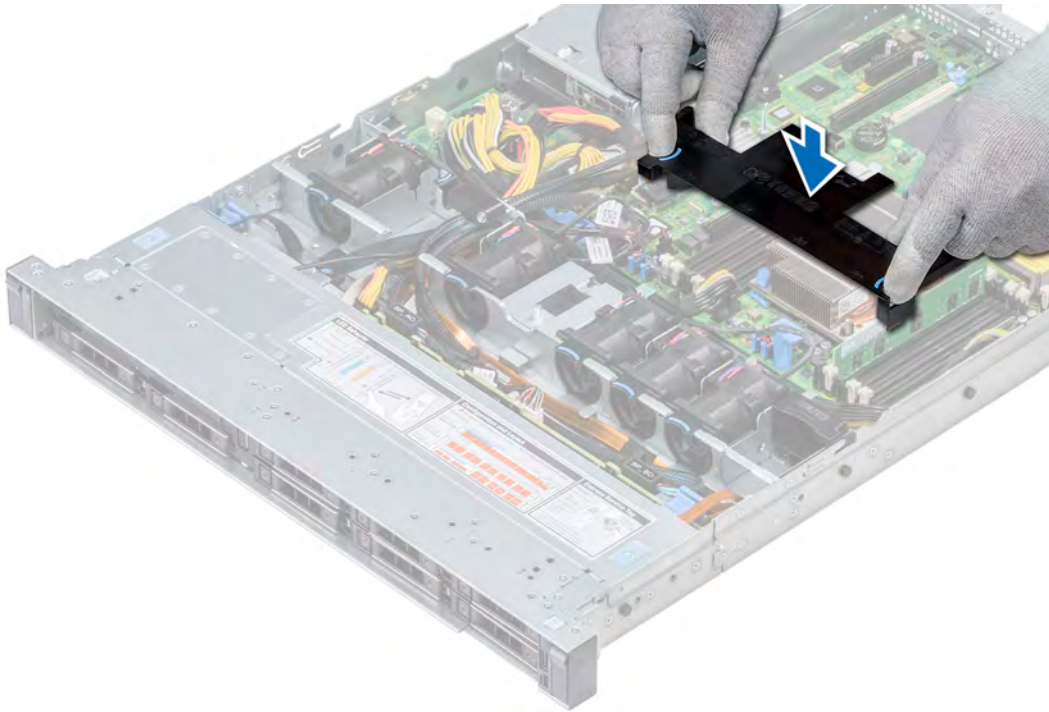
Figure 28. Installing the air shroud
