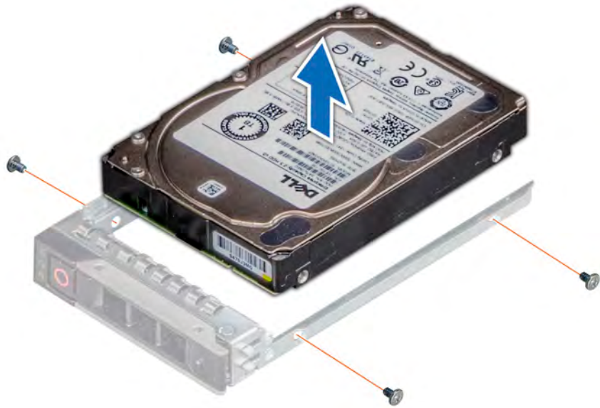
Figure 47. Removing the drive from the drive carrier
