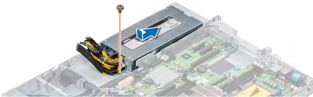
Figure 88. Installing a non-redundant cabled AC PSU
