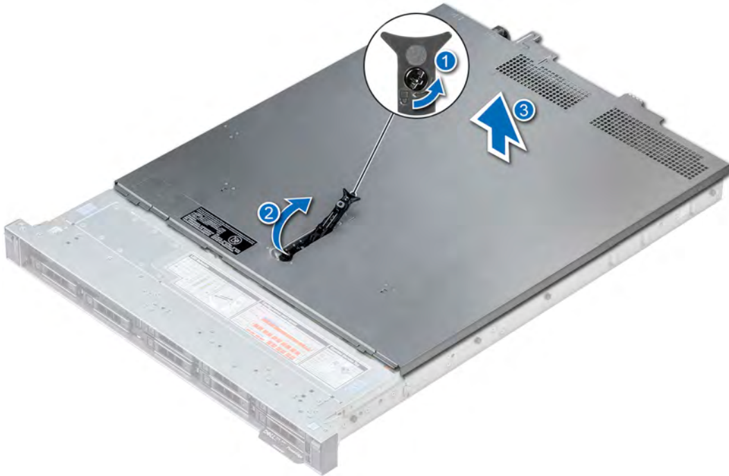
Figure 23. Removing the system cover
