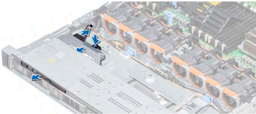
Figure 96. Removing optical drive
