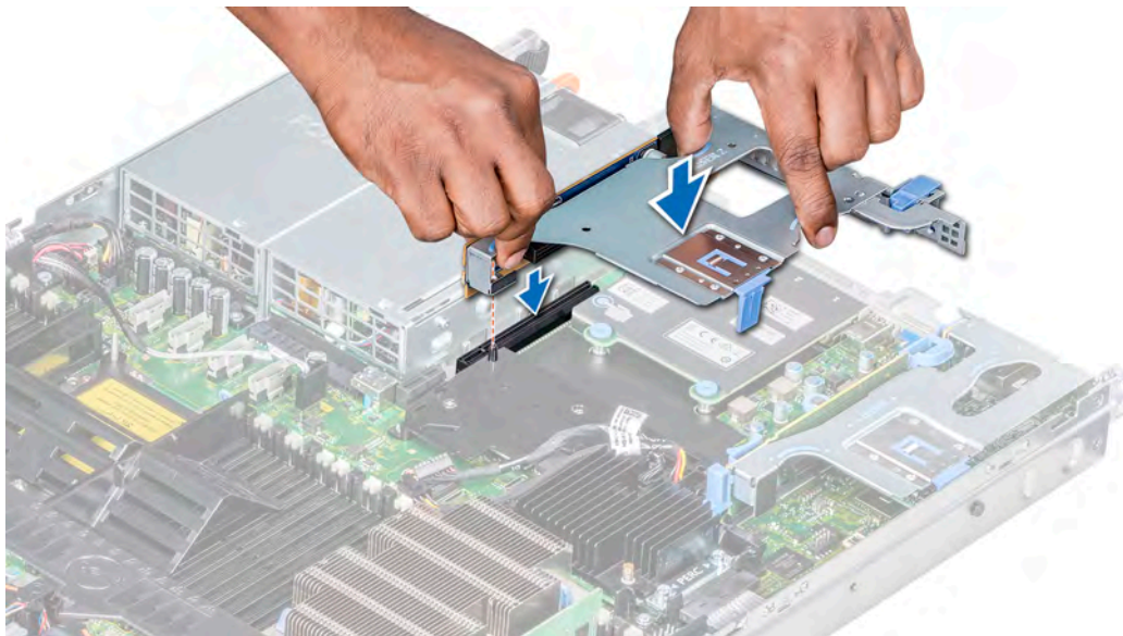
Figure 51. Installing the expansion riser 2B
