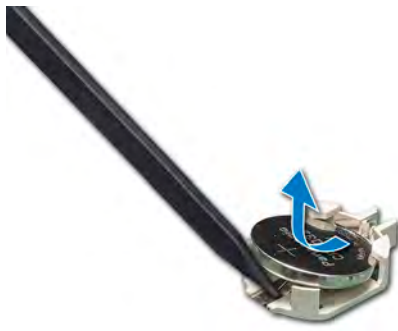
Figure 92. Removing the system battery
