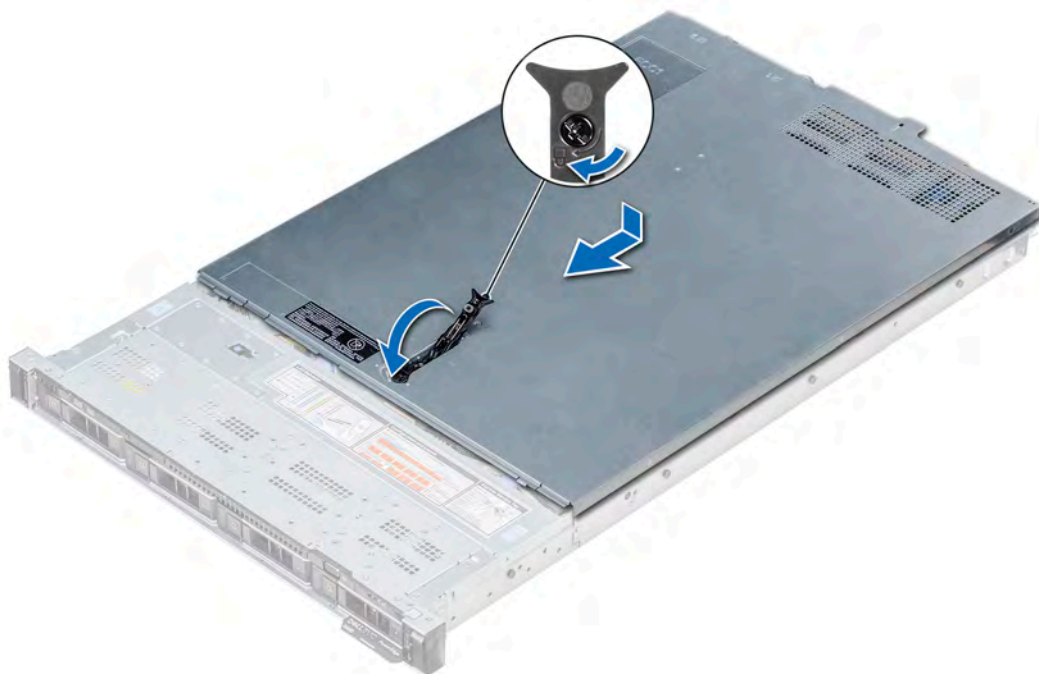
Figure 22. Installing the system cover
