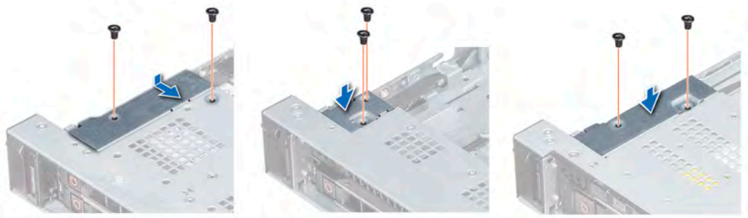
Figure 108. Installing the cable cover
