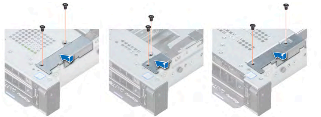
Figure 112. Installing the cable cover
