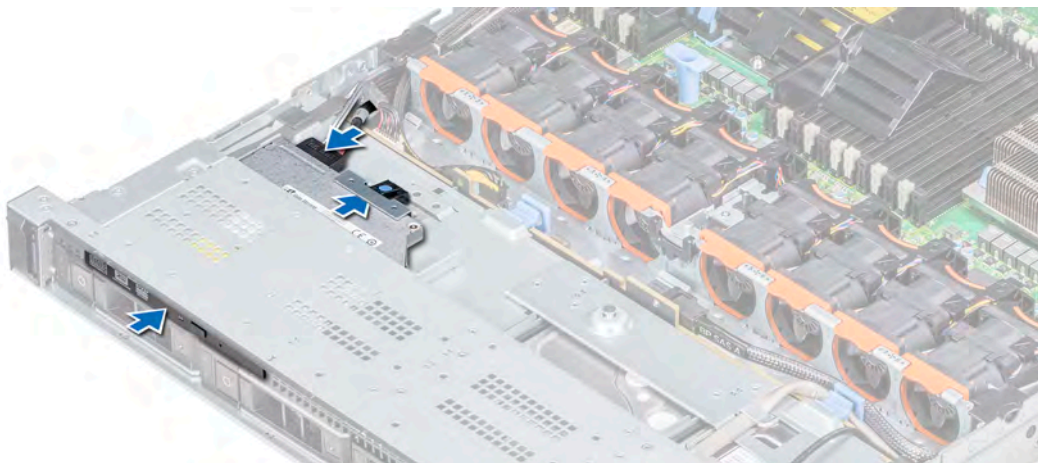
Figure 97. Installing the optical drive
