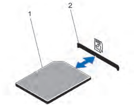
Figure 43. Removing and Installing the SD vFlash Card
