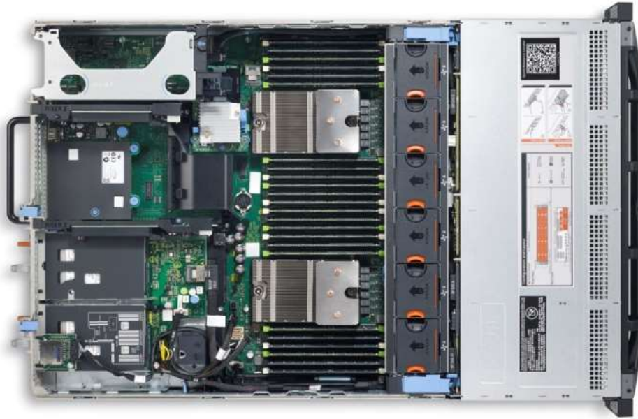
Figure 8. R720xd internal chassis view
