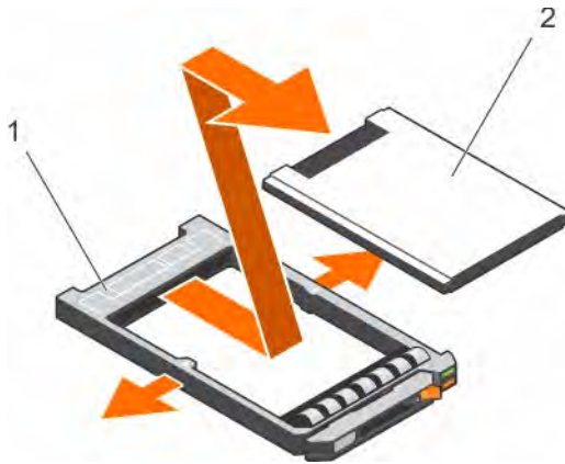
Figure 96. Removing a 1.8-inch hard drive into a hard drive carrier
