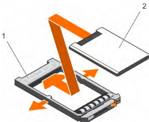
Figure 97. Installing a 1.8-inch hard drive into a hard drive carrier
