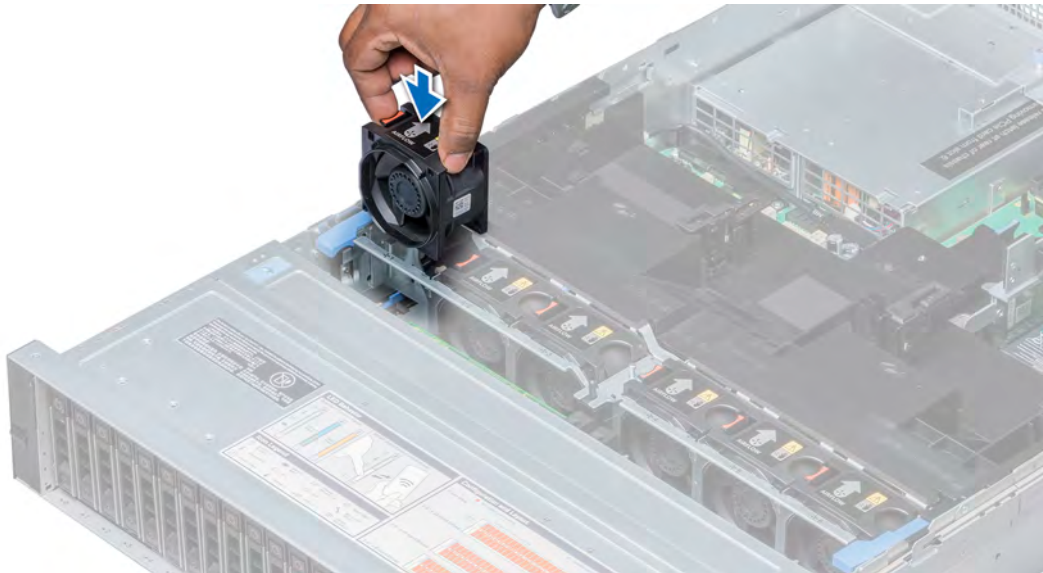
Figure 36. Installing cooling fan
