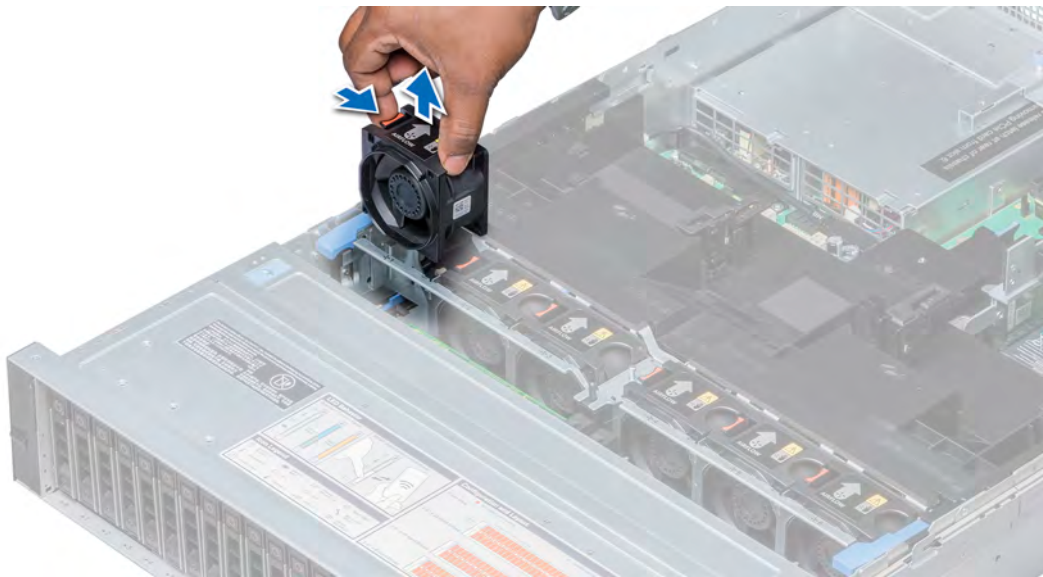
Figure 35. Removing cooling fan
