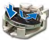
Figure 121. Installing the system battery
