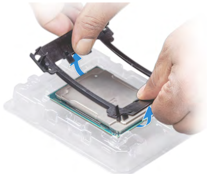
Figure 59. Removing the processor bracket
