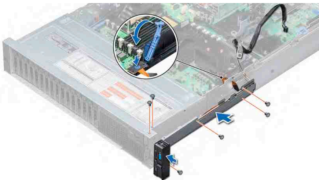
Figure 141. Installing right control panel
