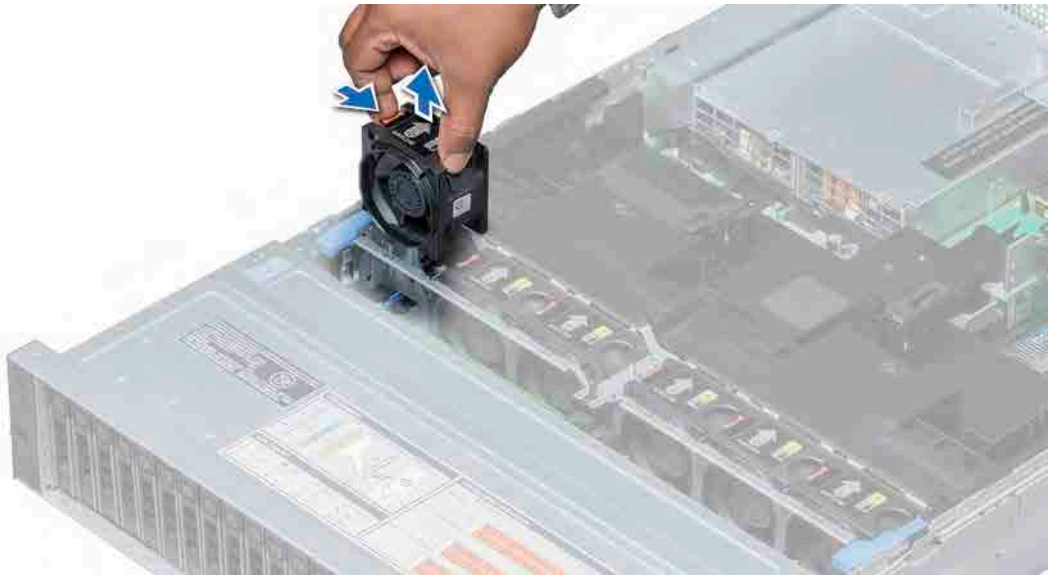
Figure 29. Removing cooling fan
