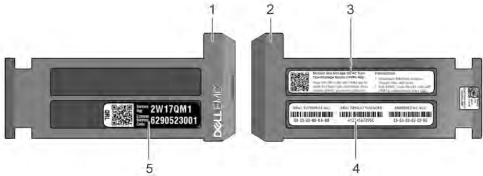
Figure 15. Locating Service Tag of your system
