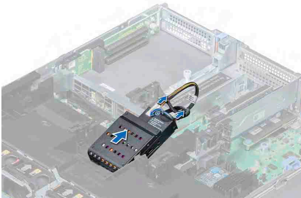
Figure 33. Removing the NVDIMM-N battery from the air shroud
