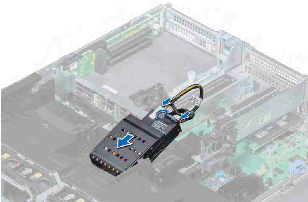
Figure 34. Installing NVDIMM-N battery into air shroud
