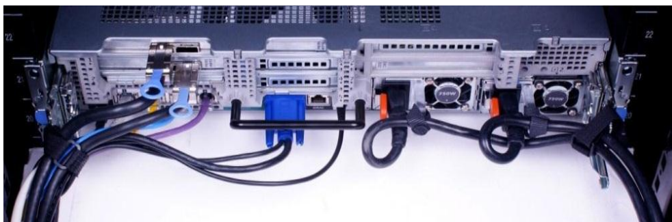
Figure 9. Cable routing without a CMA
