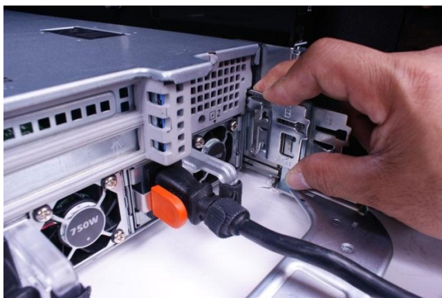
Figure 3. Attaching the inner CMA attachment bracket
