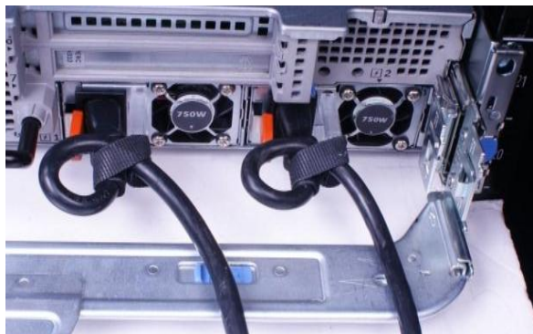
Figure 2. Routing power cables through the strain reliefs
