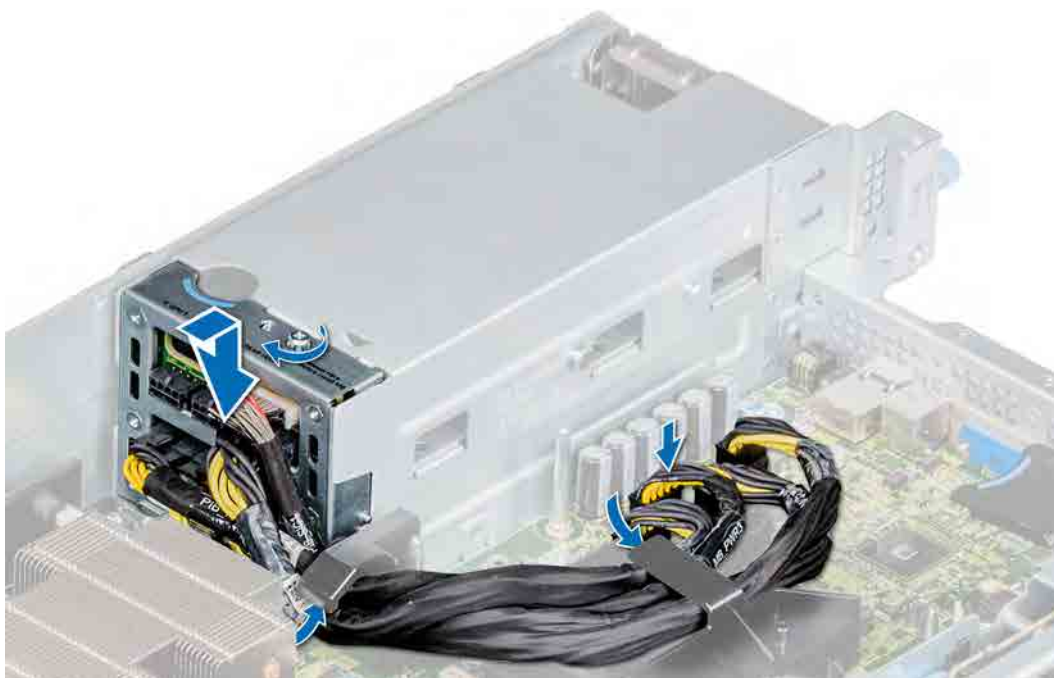
Figure 109. Installing power interposer board
