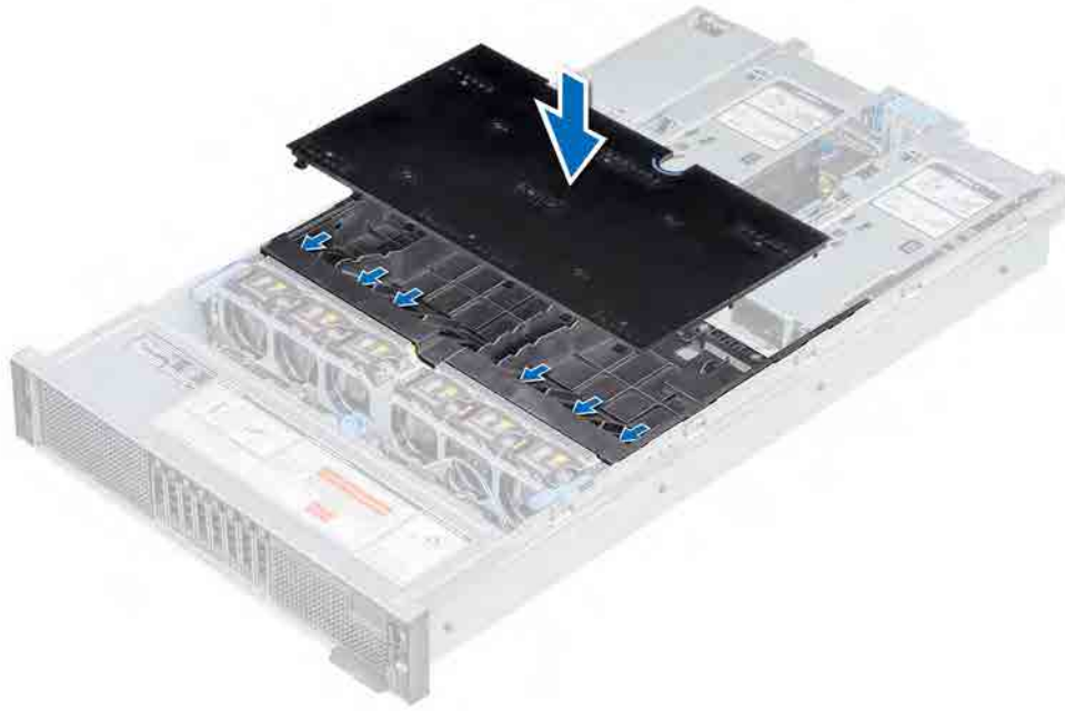
Figure 26. Installing the GPU air shroud cover
