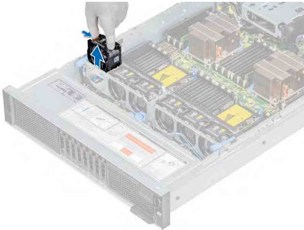
Figure 29. Removing cooling fan
