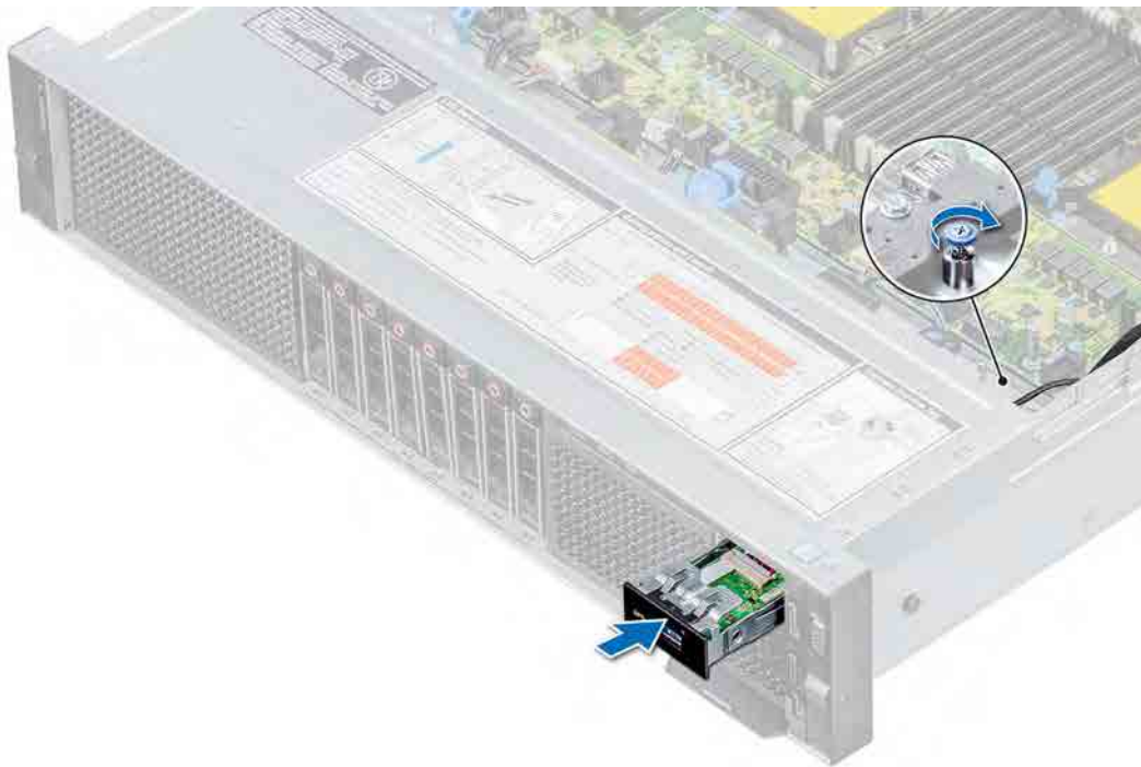
Figure 101. Installing USB 3.0 module
