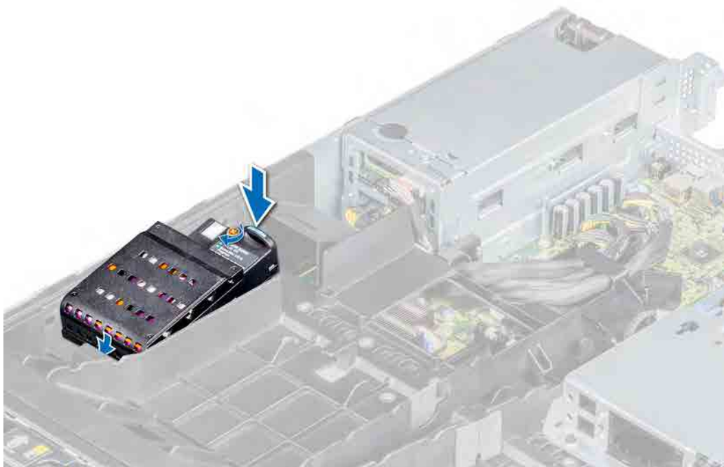
Figure 34. Installing NVDIMM-N battery into GPU air shroud
