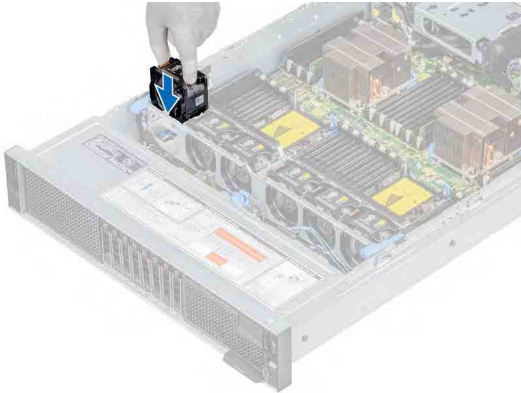
Figure 30. Installing cooling fan
