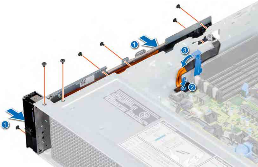
Figure 114. Installing left control panel
