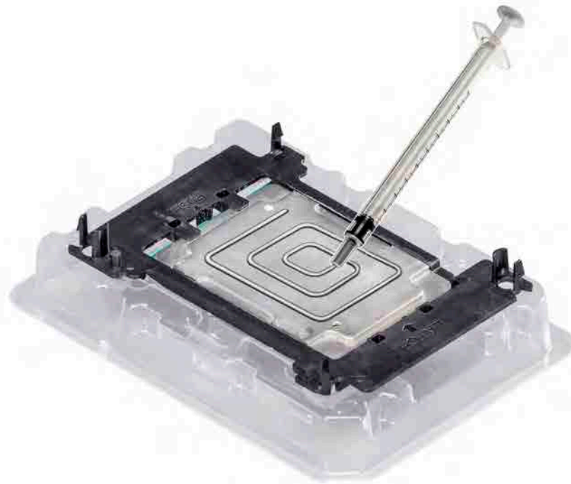
Figure 71. Applying thermal grease on top of the processor
