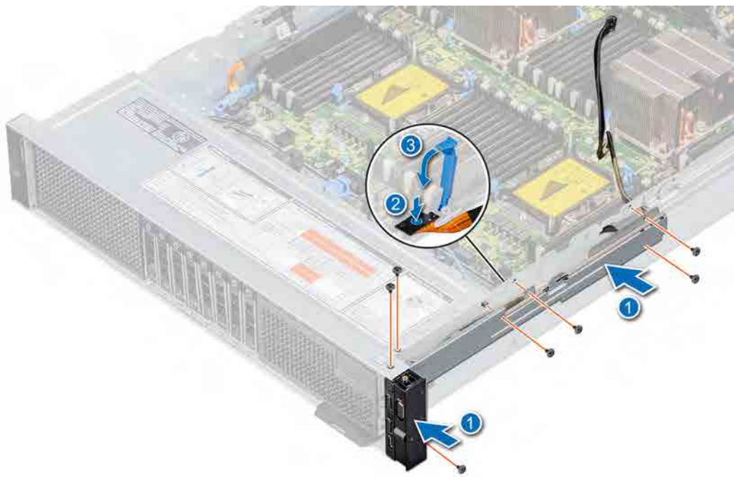
Figure 116. Installing right control panel
