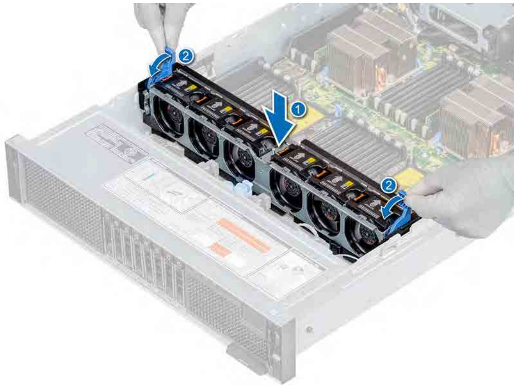
Figure 28. Installing the cooling fan assembly
