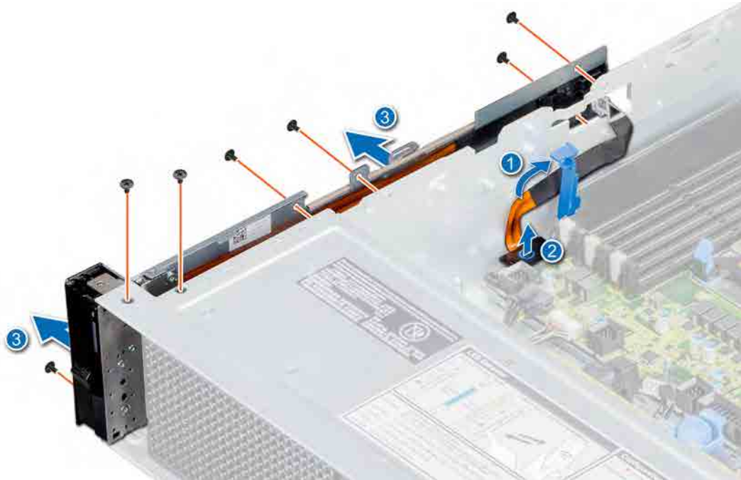
Figure 113. Removing left control panel
