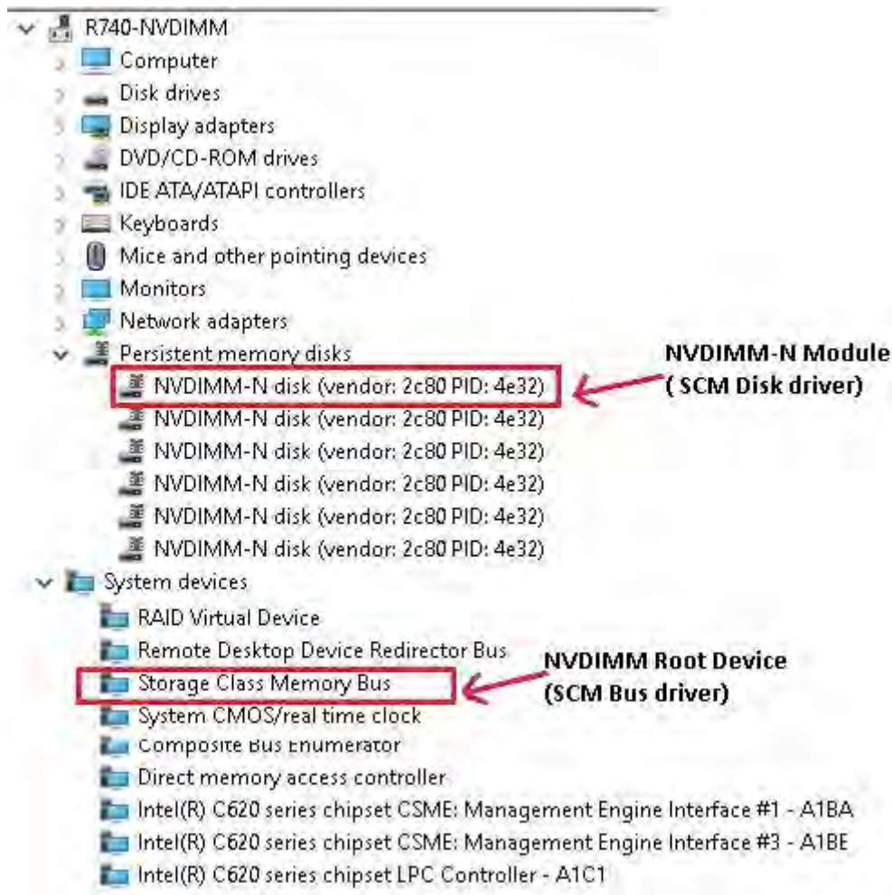
Figure 18. Windows device manager view of NVDIMM-N root device and NVDIMM-N disk instances
