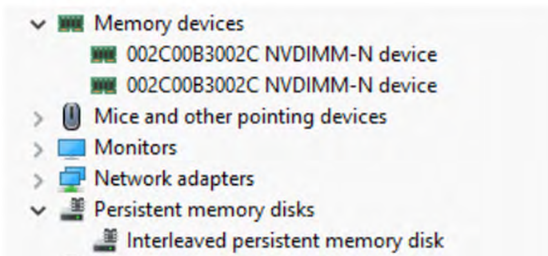
Figure 29. Interleaved Persistent Memory Disk in Device Manager
