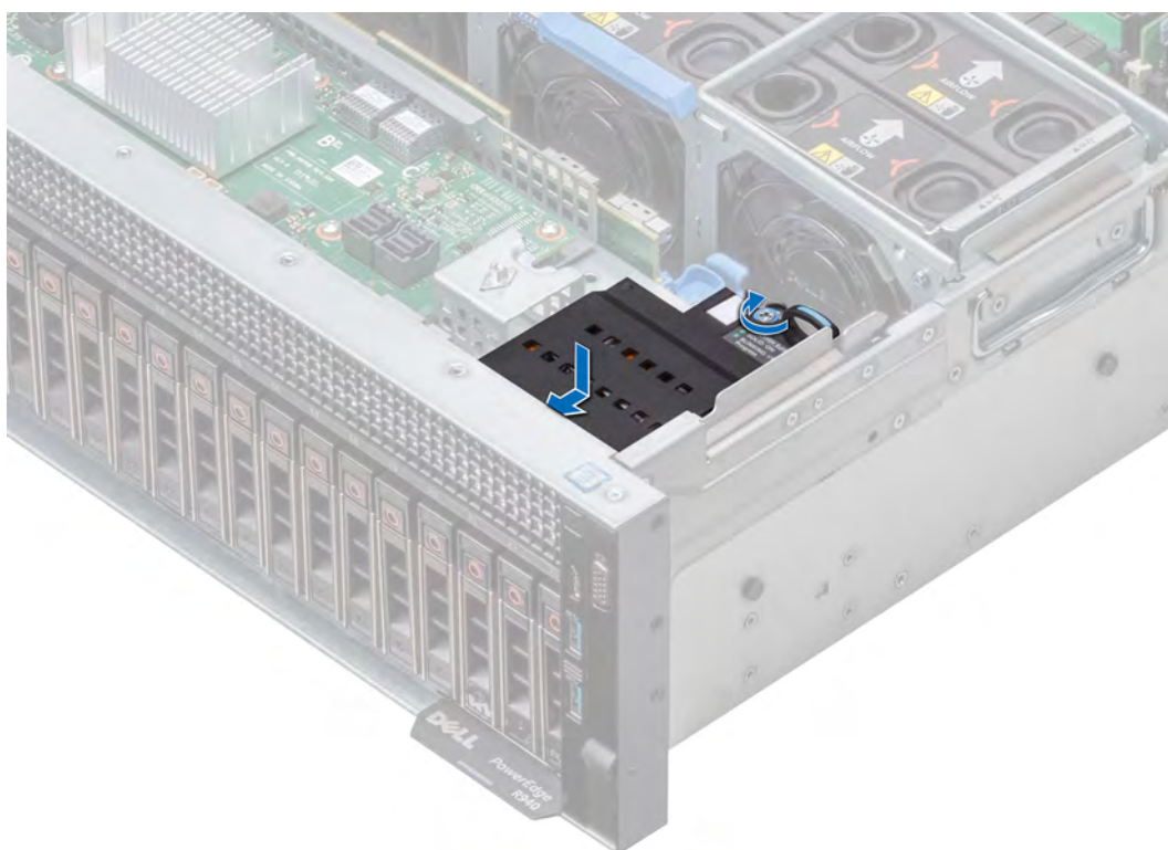
Figure 99. Installing NVDIMM-N battery
