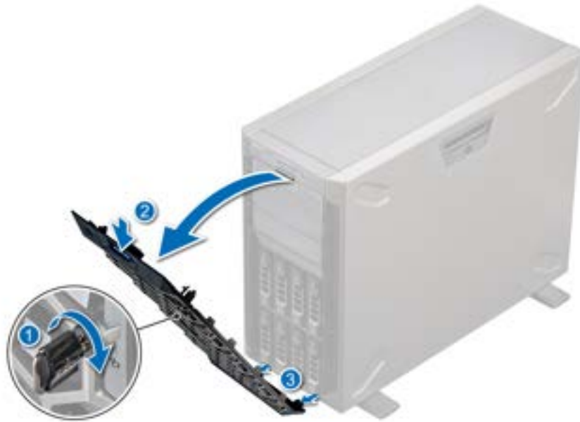
Figure 17. Removing the front bezel
