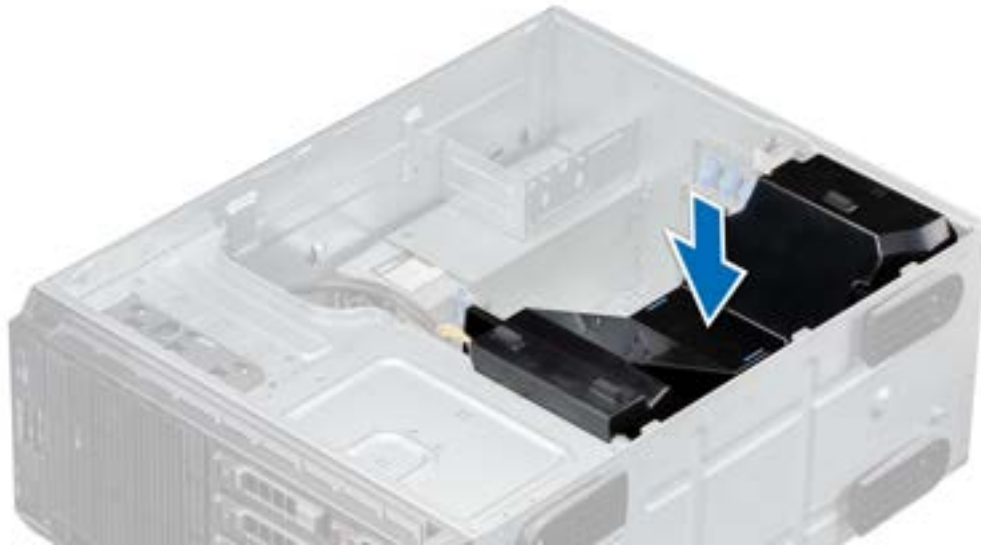
Figure 25. Installing the air shroud
