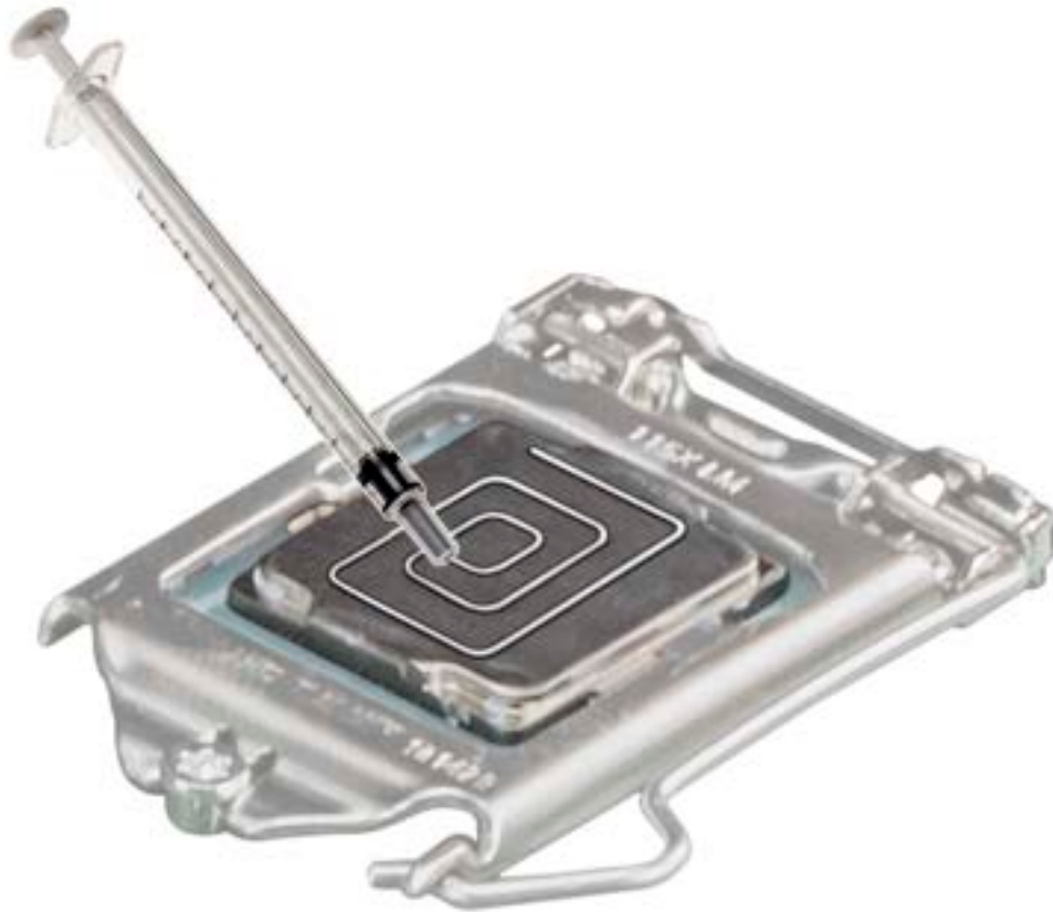
Figure 68. Applying thermal grease on top of the processor
