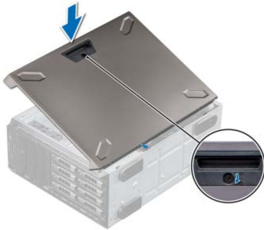
Figure 23. Installing the system cover
