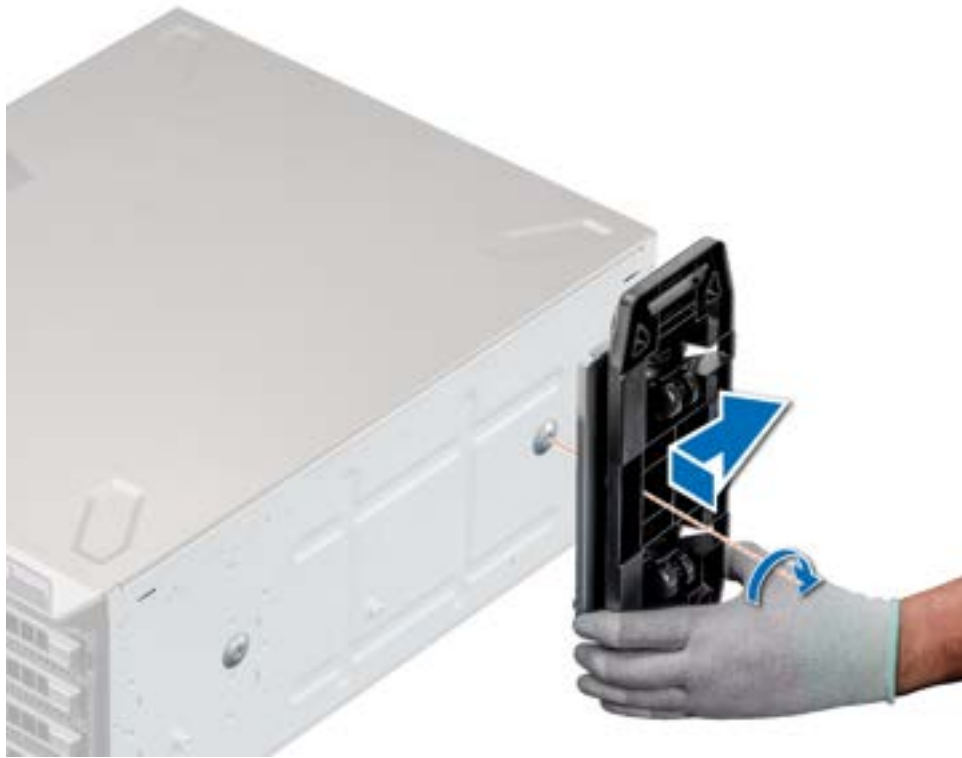
Figure 21. Installing caster wheels
