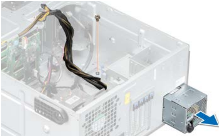
Figure 74. Removing a cabled power supply unit
