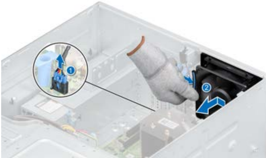
Figure 54. Removing the internal cooling fan
