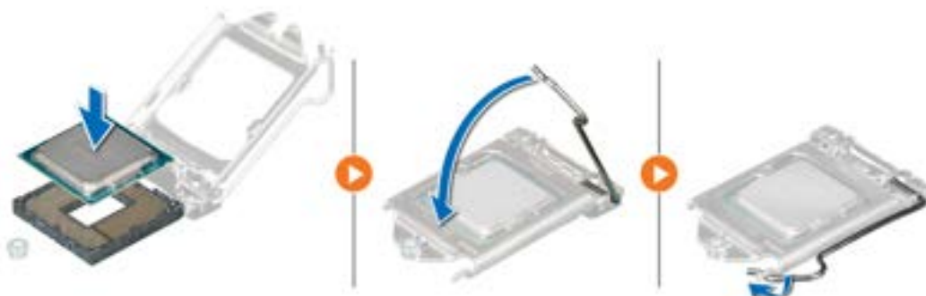
Figure 67. Installing the processor
