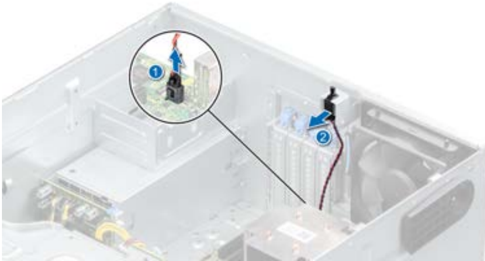
Figure 26. Removing the intrusion switch
