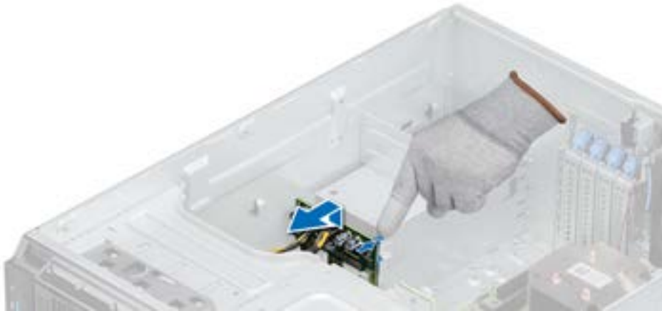
Figure 76. Removing the power interposer board
