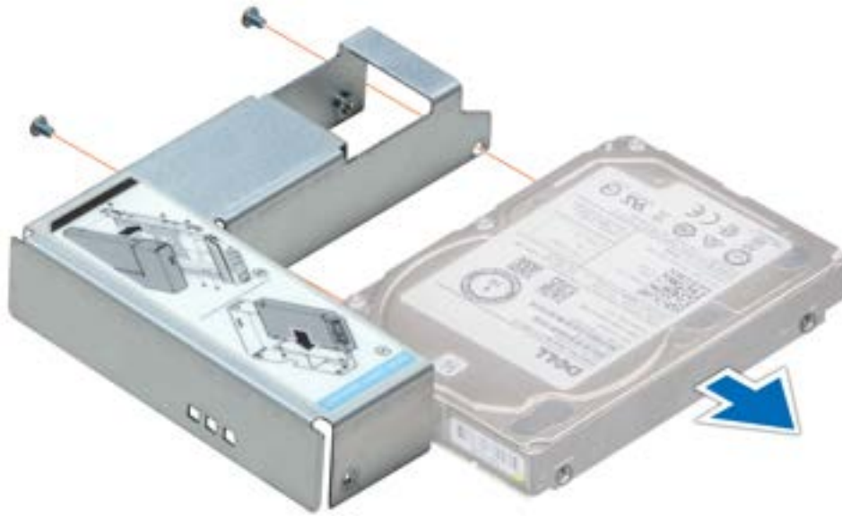
Figure 34. Removing a 2.5-inch drive from the 3.5-inch drive adapter
