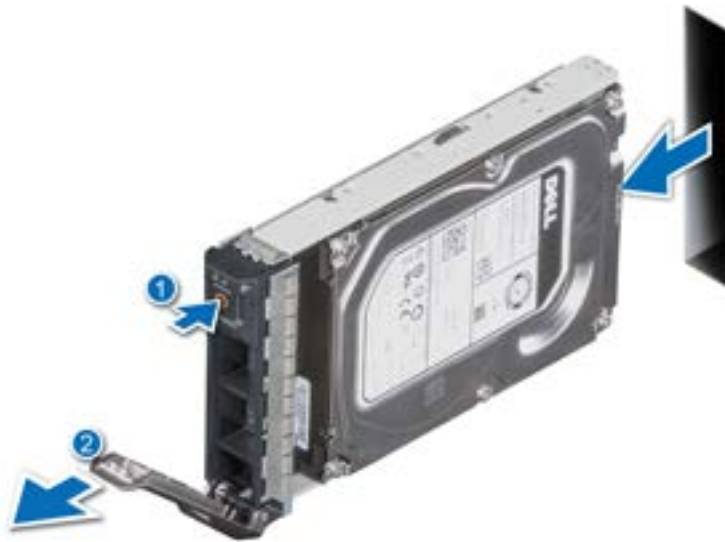
Figure 30. Removing a drive carrier
