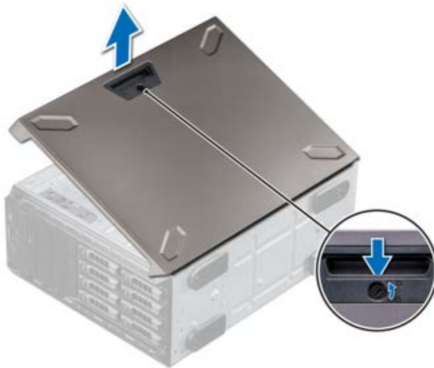
Figure 22. Removing the system cover
