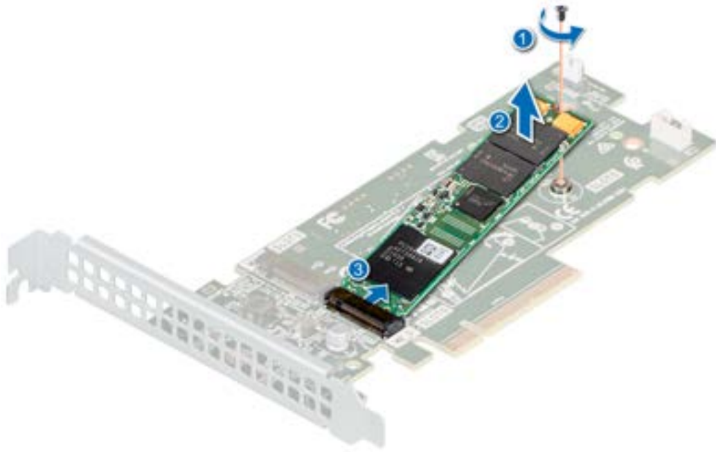
Figure 60. Removing the M.2 SSD module
