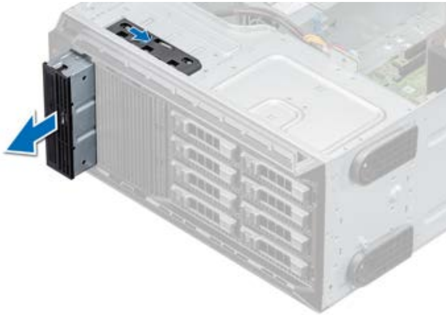
Figure 40. Removing the optical drive
