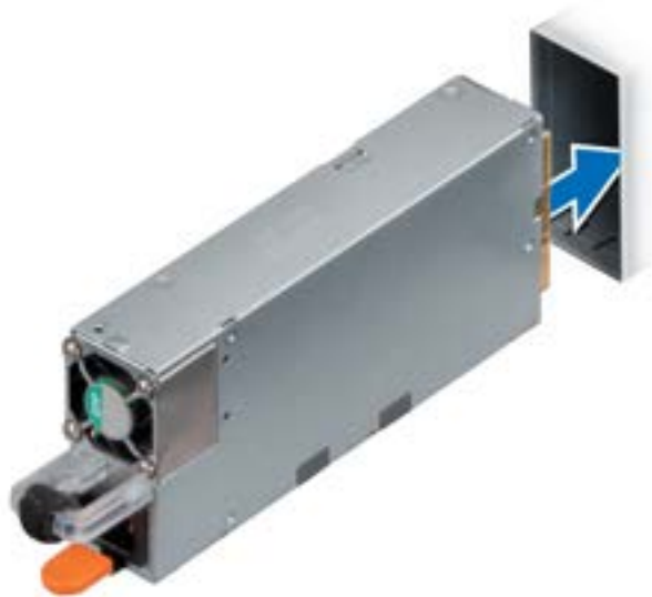
Figure 73. Installing a redundant power supply unit
