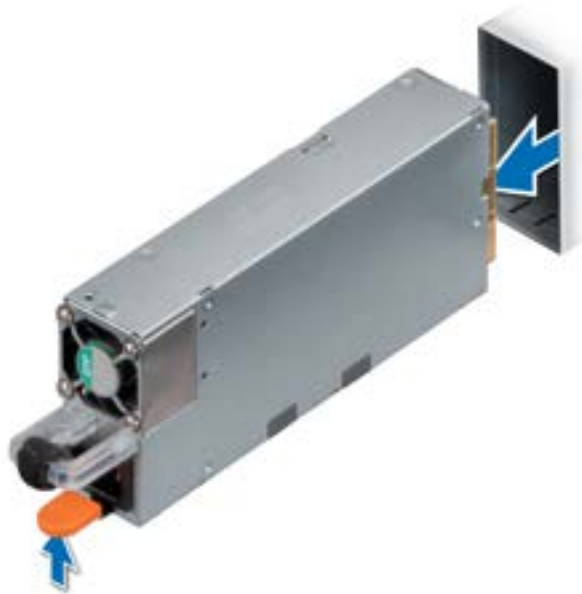
Figure 72. Removing a redundant power supply unit
