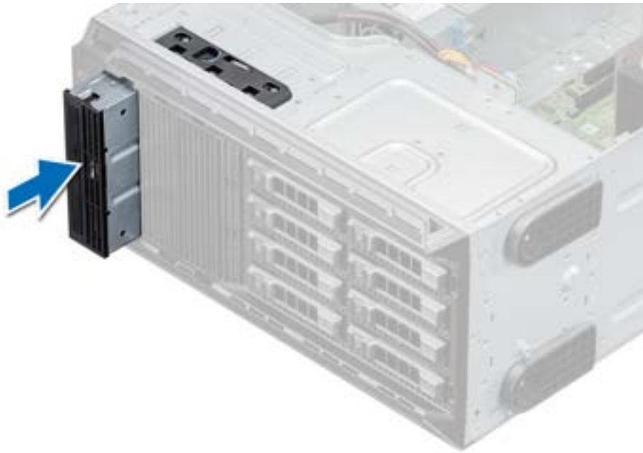
Figure 41. Installing the optical drive
