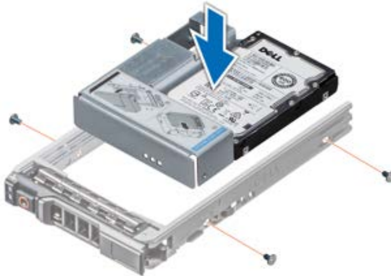
Figure 37. Installing a 3.5-inch drive adapter into the 3.5-inch drive carrier
