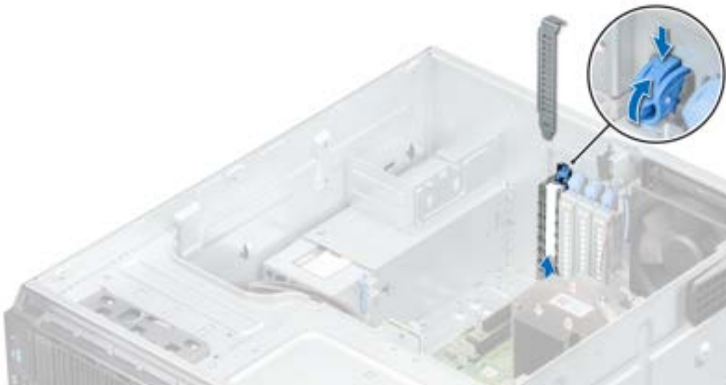
Figure 57. Removing the filler bracket
