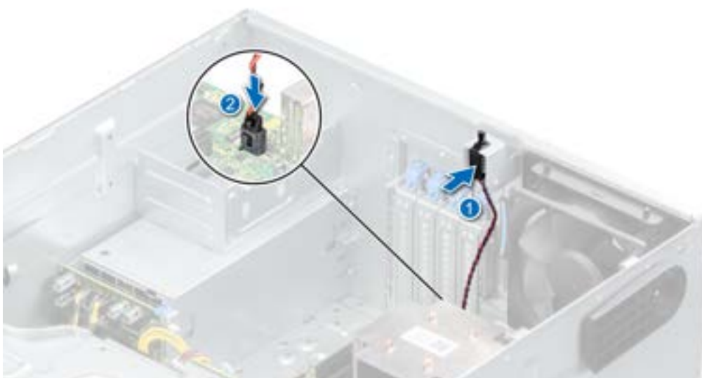
Figure 27. Installing the intrusion switch
