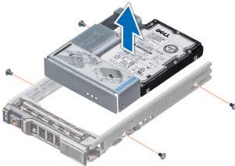
Figure 36. Removing a 3.5-inch drive adapter from a 3.5-inch drive carrier
