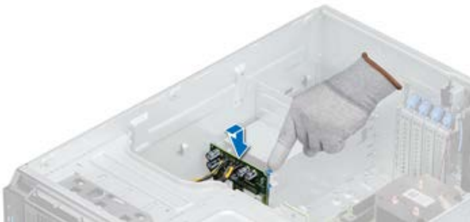
Figure 77. Installing the power interposer board
