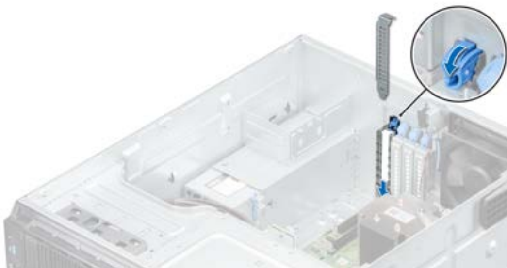
Figure 59. Installing the filler bracket
