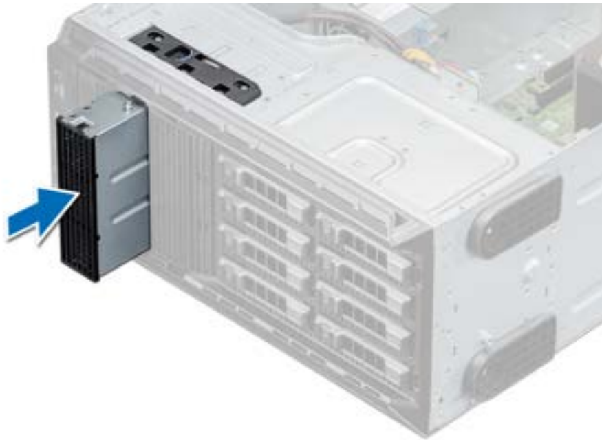
Figure 39. Installing the optical or tape drive blank
