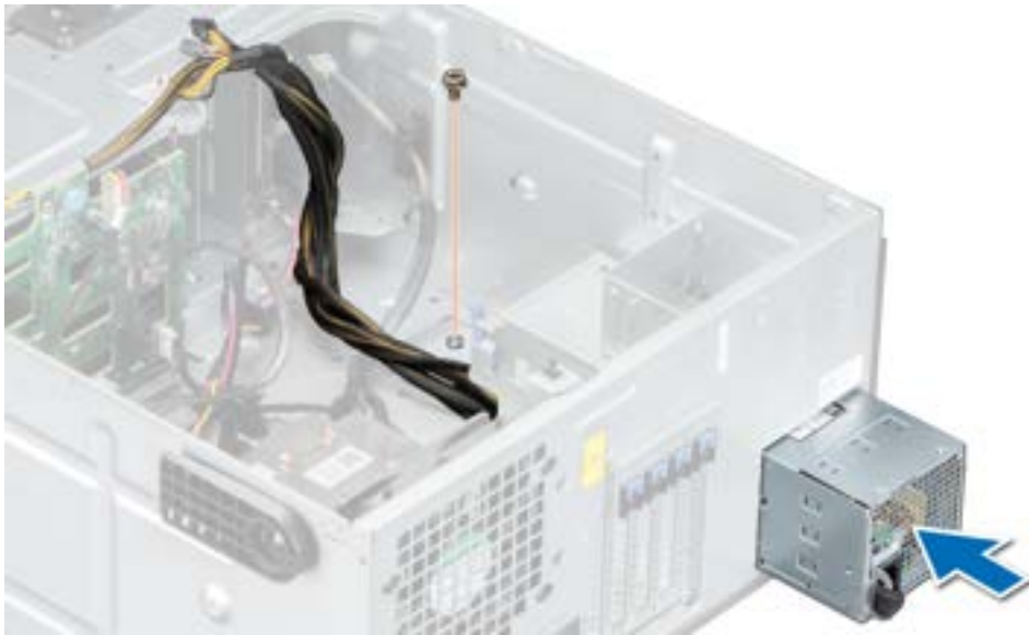
Figure 75. Installing a cabled power supply unit
