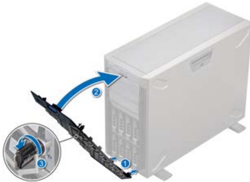
Figure 18. Installing the front bezel
