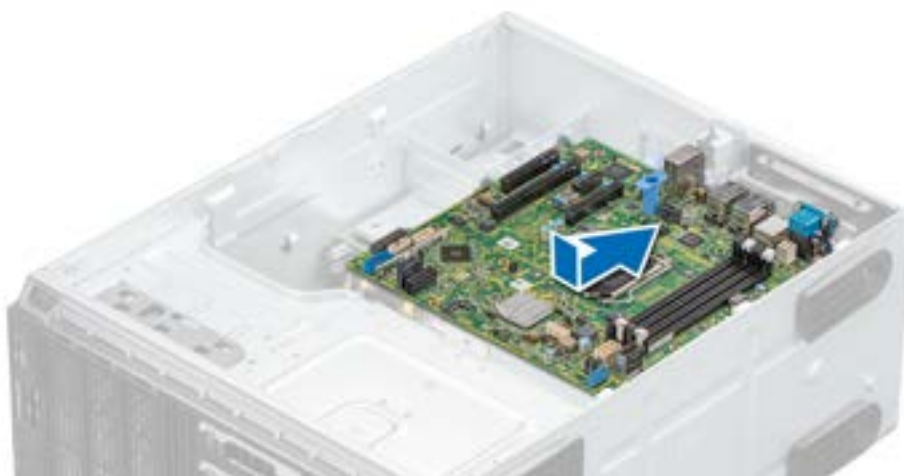
Figure 82. Installing the system board
