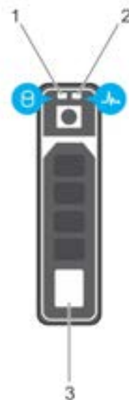
Figure 91. Drive indicators on the drive and the mid drive tray backplane
