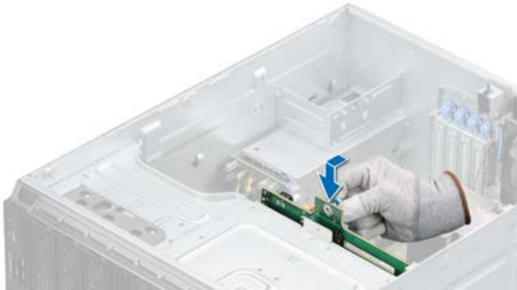
Figure 46. Installing the drive backplane
