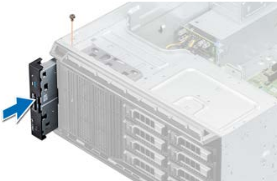
Figure 85. Installing the control panel
