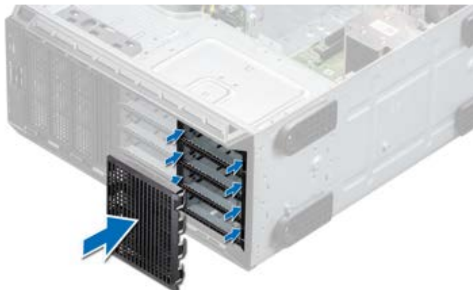
Figure 50. Installing a four-slot drive blank
