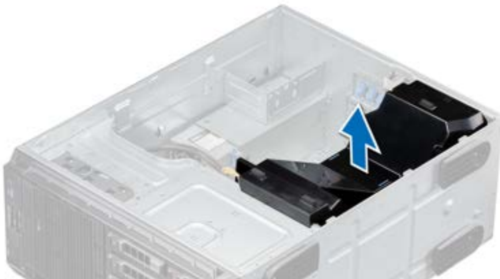
Figure 24. Removing the air shroud
