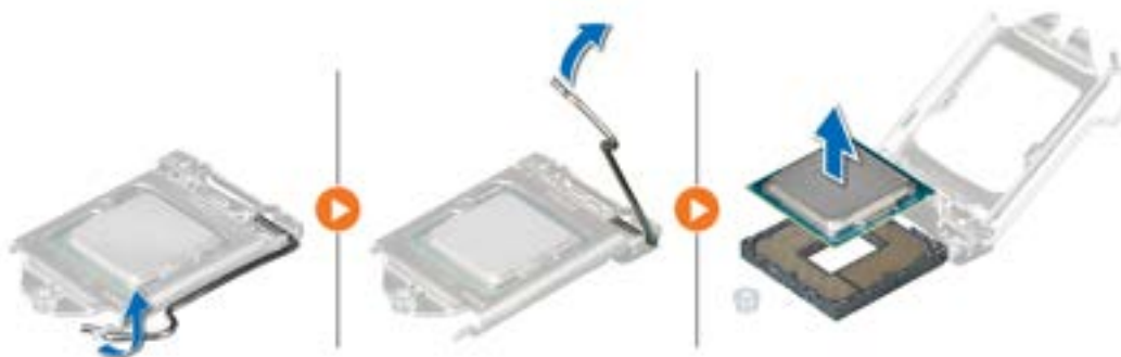
Figure 66. Removing the processor
