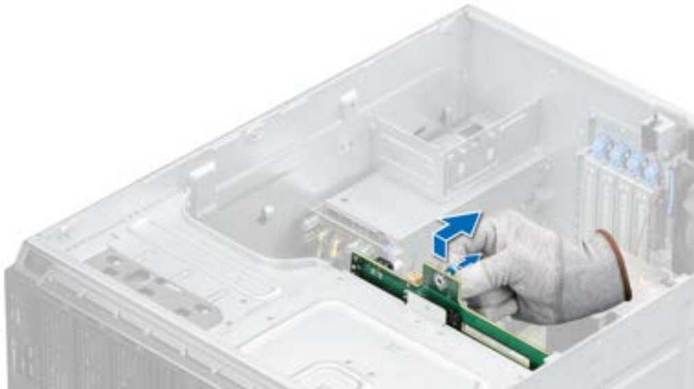
Figure 45. Removing the drive backplane
