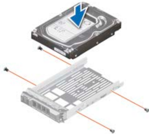
Figure 33. Installing a drive into the drive carrier
