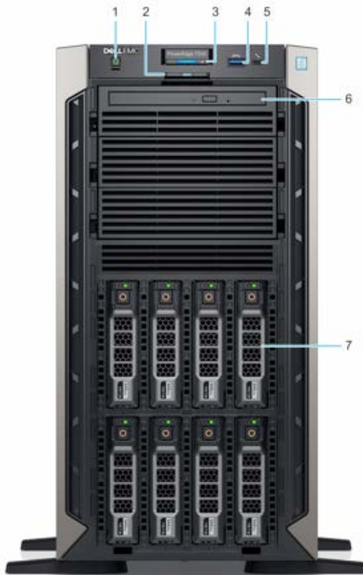
Figure 1. Front view of 8 x 3.5-inch drive system
