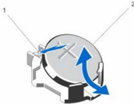
Figure 57. Removing and Installing the System Battery
