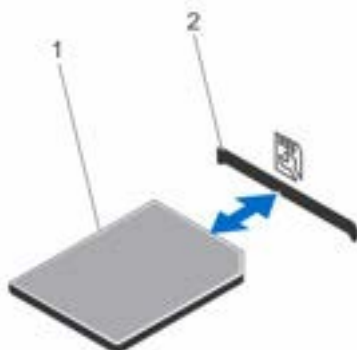
Figure 48. Removing and Installing the SD vFlash Card
