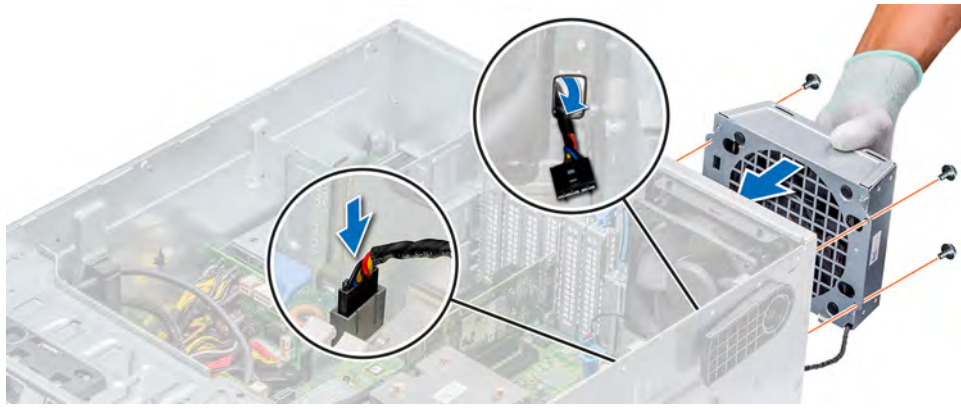
Figure 55. Installing the external cooling fan
