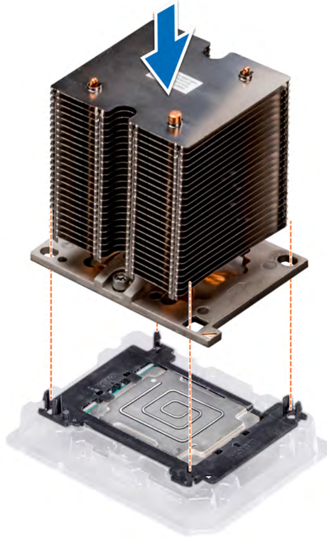
Figure 69. Installing the heat sink onto the processor
