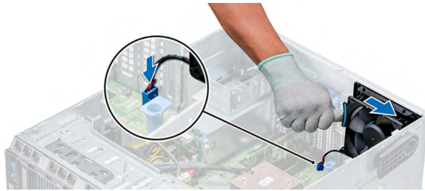
Figure 53. Installing the internal cooling fan
