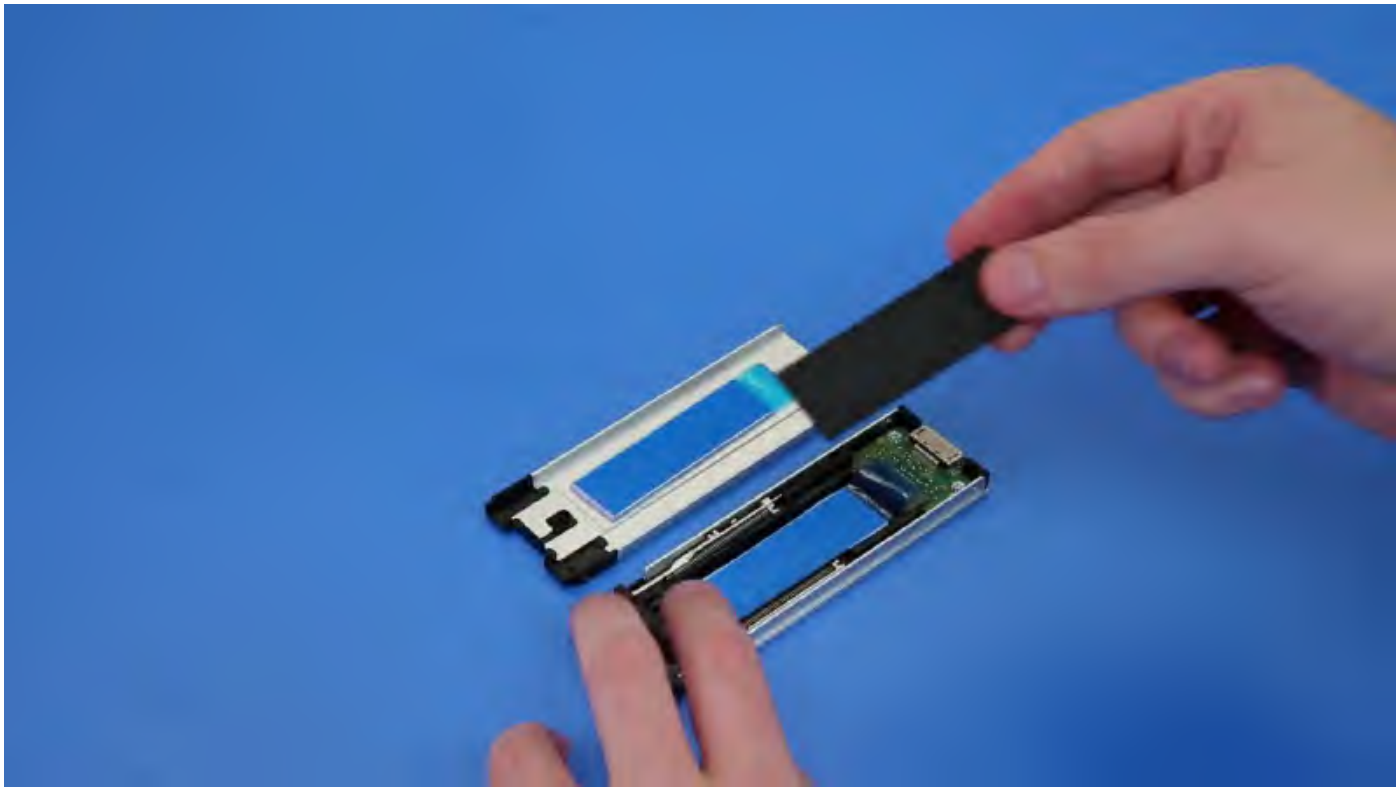
b. Peel off the tape from the SSD carrier.
