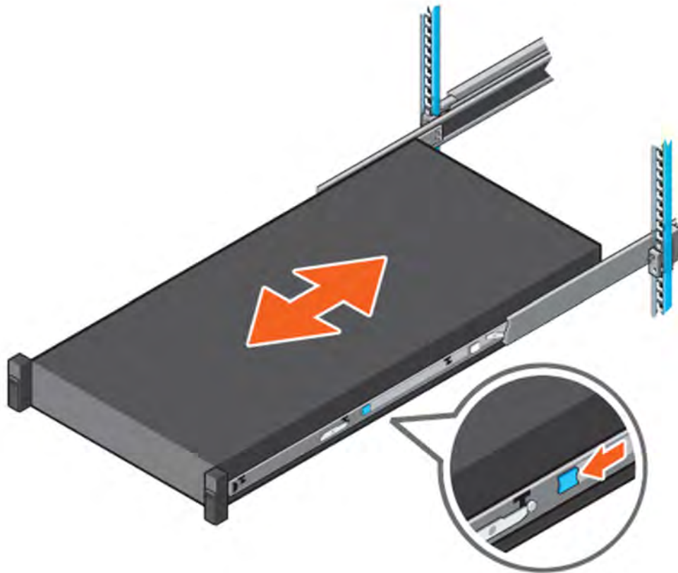
Figure 27. Slide system into the rack
