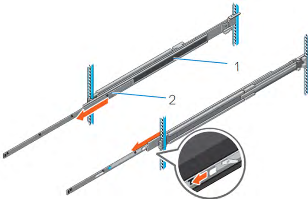
Figure 28. Pull out the intermediate rail
