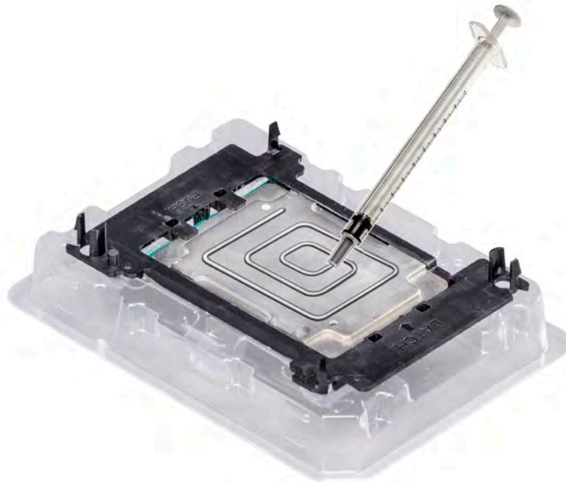
Figure 15. Applying thermal grease on top of the processor
