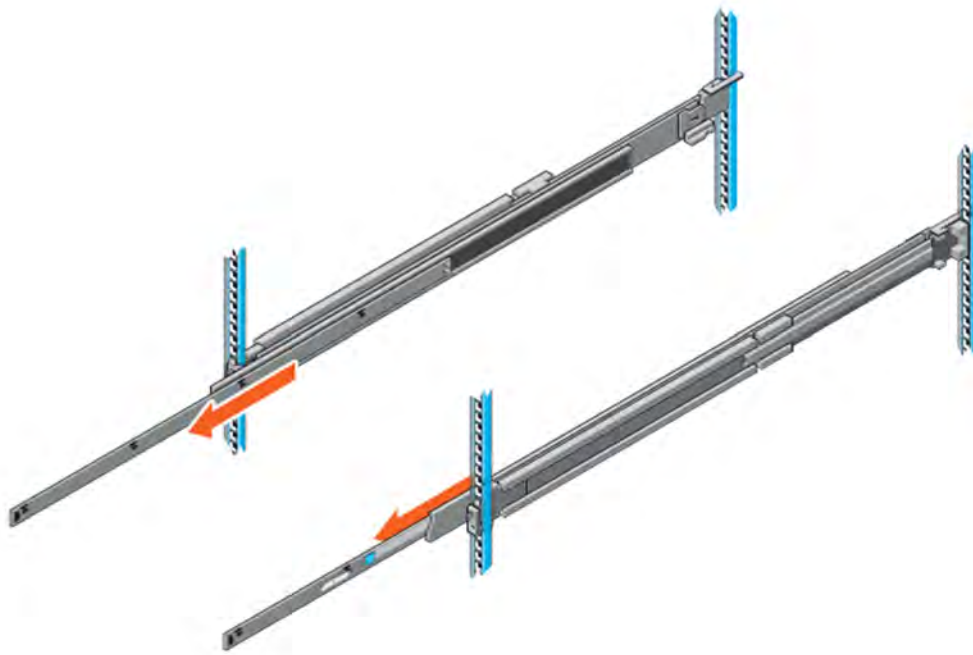
Figure 25. Pull out inner rail
