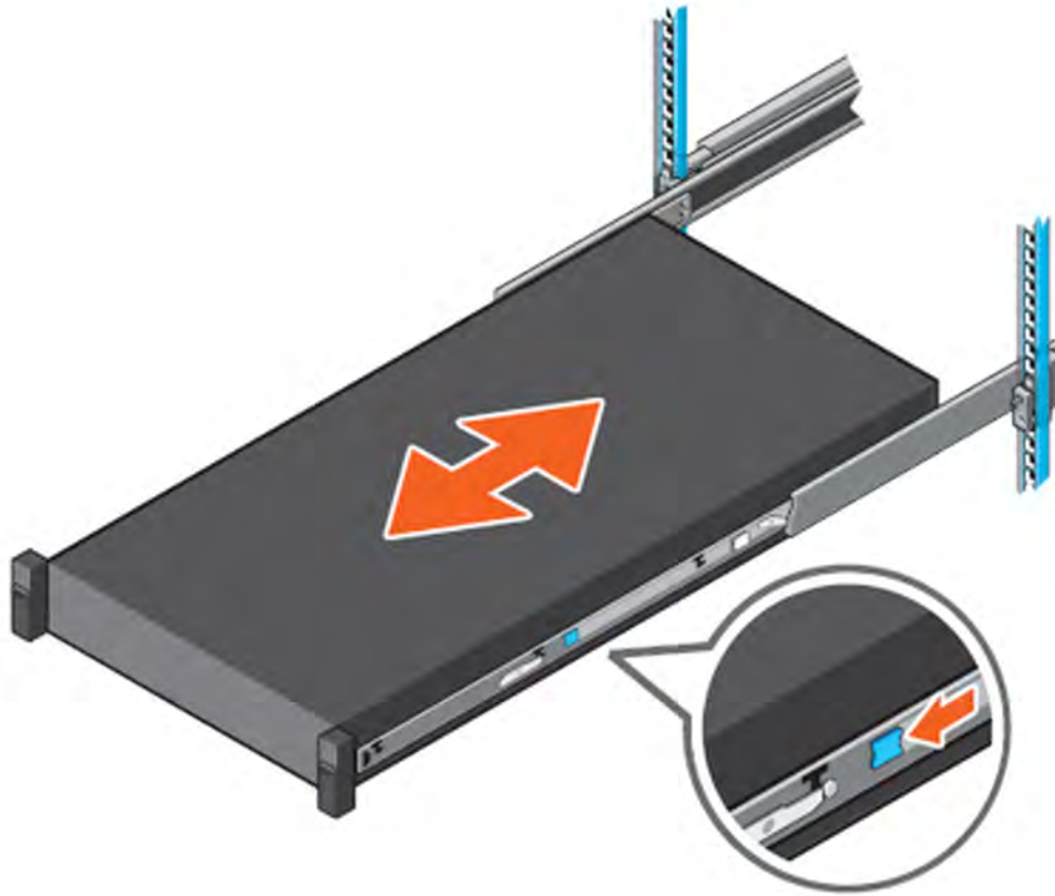
Figure 31. Slide system into the rack
