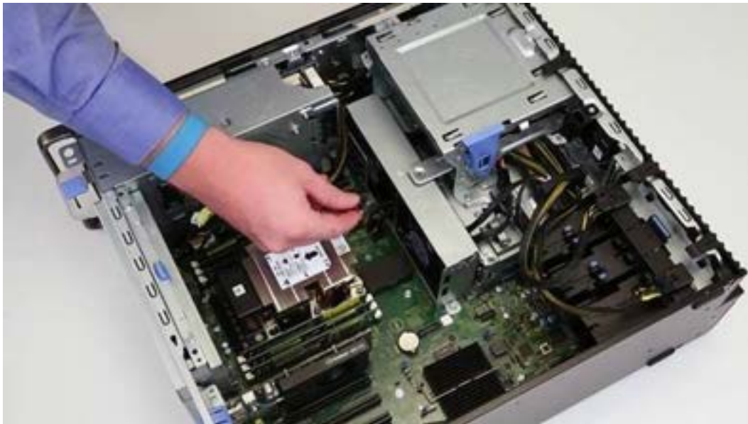
c. Tighten the heatsink screws to the system board
