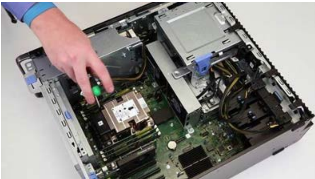
d. Remove the cap from the CPU 1 connector(in upgrading scenarios)
