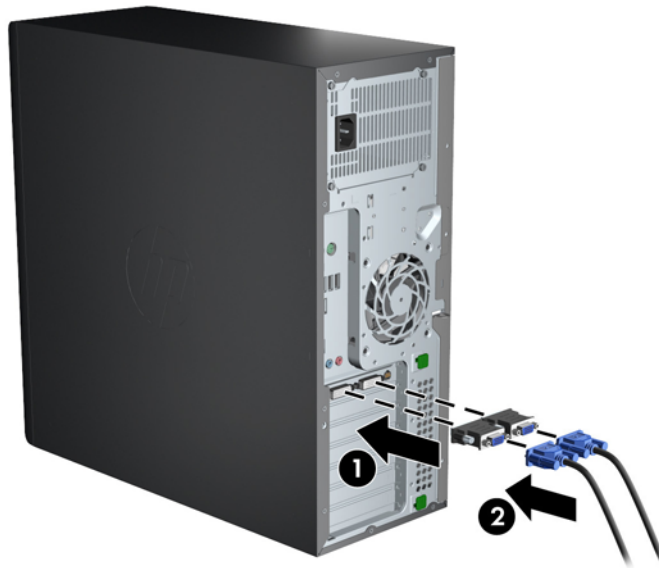
Figure 3-4 Connecting the cables to the workstation
