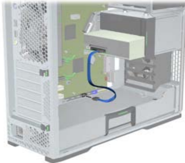
Figure 10-6 Connecting the ODD data cable to the system board
