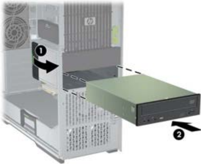
Figure 10-4 Installing the optical drive
