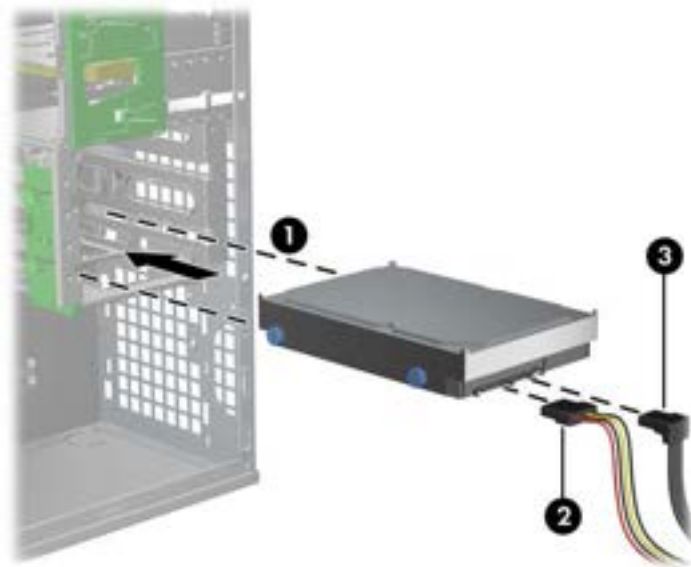
Figure 9-4 Installing the HDD drive
