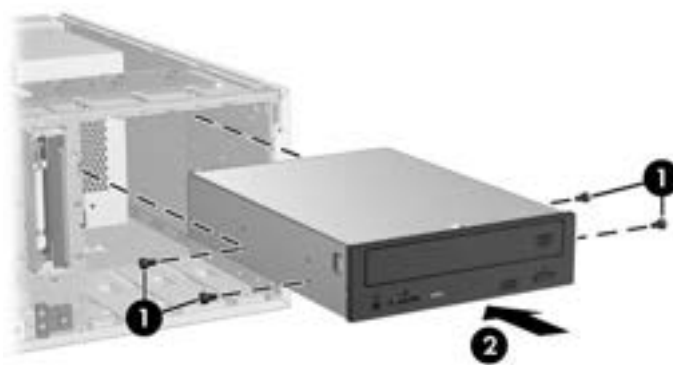
Figure 10-3 Installing the optical drive
