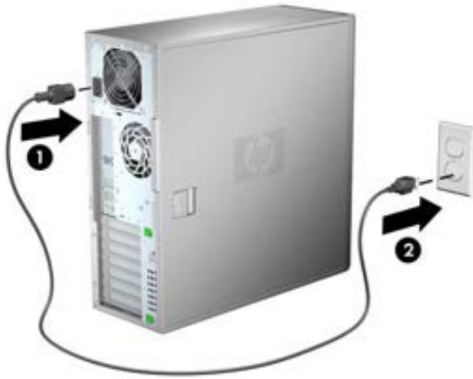
Figure 3-3 Connecting the power cord
