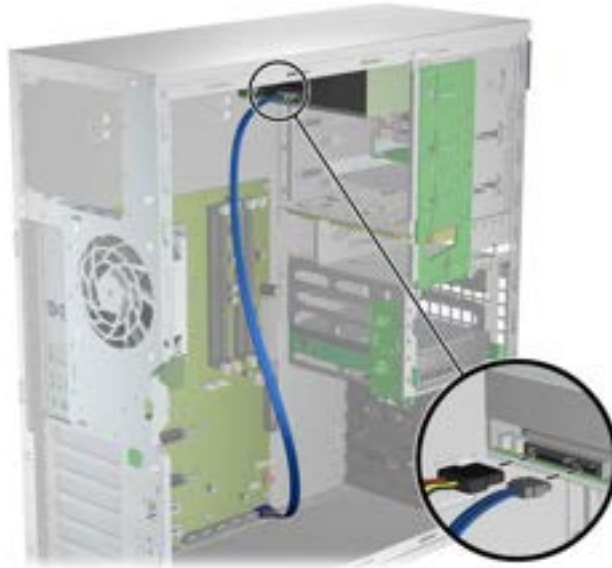
Figure 10-2 Connecting ODD power and data cables
