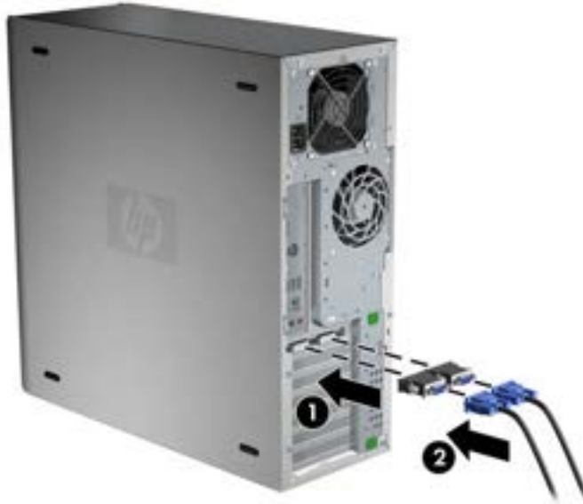
Figure 3-8 Connecting the cables to the workstation
