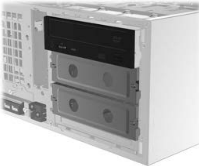
Figure 3-7 Reinstalling the optical drive
