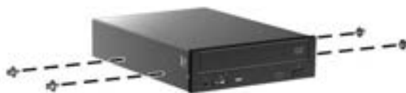
Figure 10-1 Installing the guide screws
