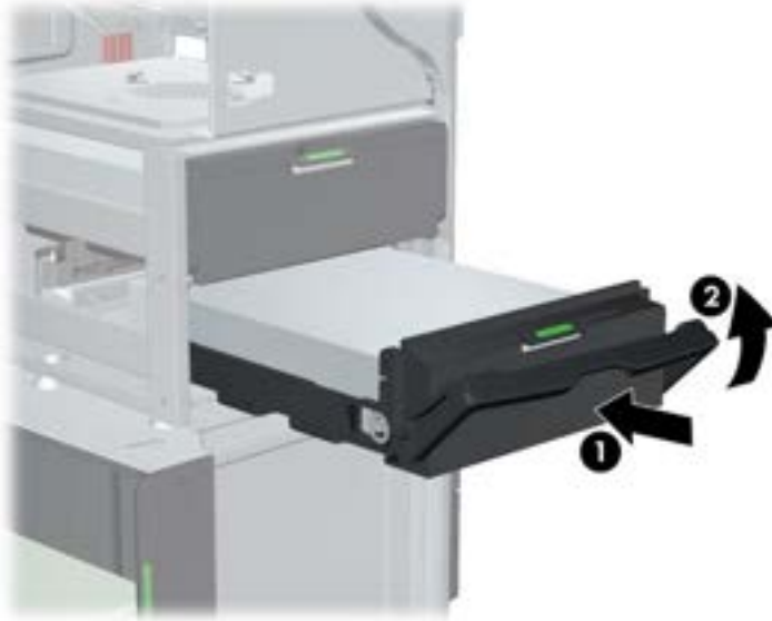
Figure 9-6 Installing the HDD in the chassis
